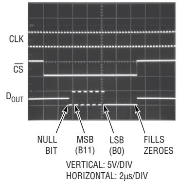
Figure 24. Scope Trace of the LTC1294/6 “Quick Look” Circuit Showing A/D Output 1010101010 (AAA<sub>HEX</sub>)
