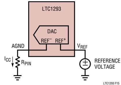
Figure 15. Parasitic Pin Resistance ( $R_{PIN}$ )
