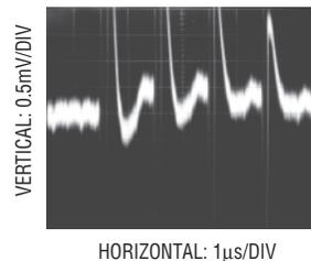
Figure 14. Poor Reference Settling Can Cause A/D Errors
