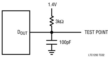
Load Circuit for  $t_{enSSO}$  and  $t_{disSSO}$
