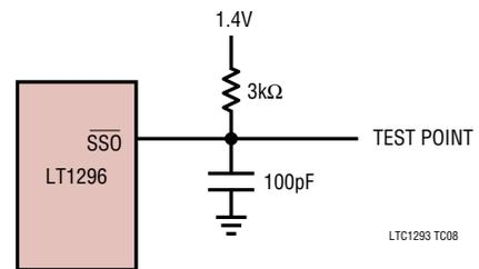
Load Circuit for  $t_{dis}$  and  $t_{en}$
