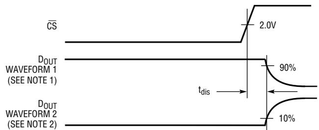
Voltage Waveform for  $D_{OUT}$  Delay Time,  $t_{dDO}$
