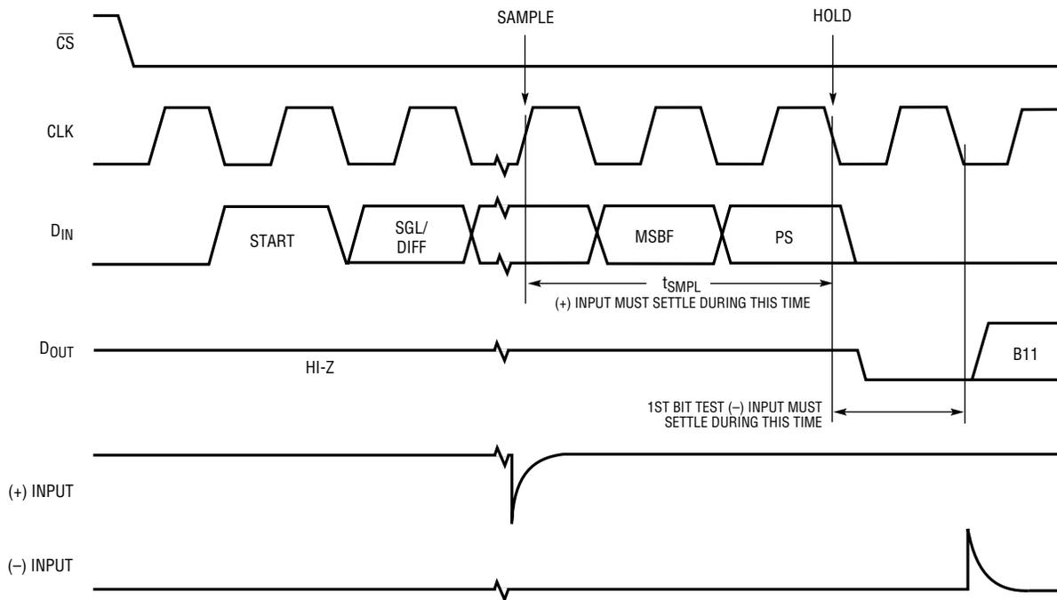
Figure 8. “+” and “-” Input Settling Windows
