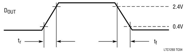
Voltage Waveform for  $t_{enSSO}$
