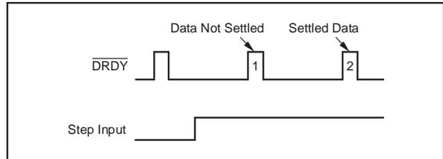
**Figure 45. Asynchronous Step-Input Settling Time (DRATE[1:0] = 10, 01, 00)**
