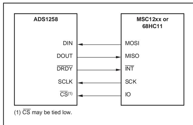
Figure 64. Connection to Microcontrollers with an SPI Interface
