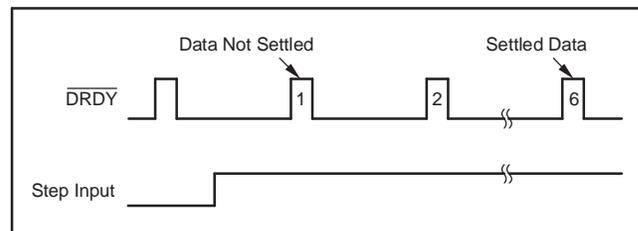
**Figure 46. Asynchronous Step-Input Settling Time (Fixed-Channel Mode, DRATE[1:0] = 11)**
