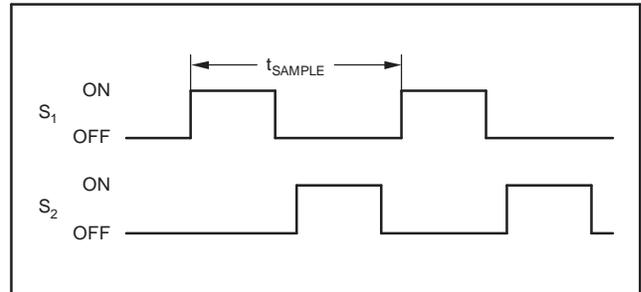
Figure 36.  $S_1$  and  $S_2$  Switch Timing for Figure 37
