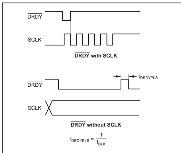
Figure 52.  $\overline{\text{DRDY}}$  Timing
