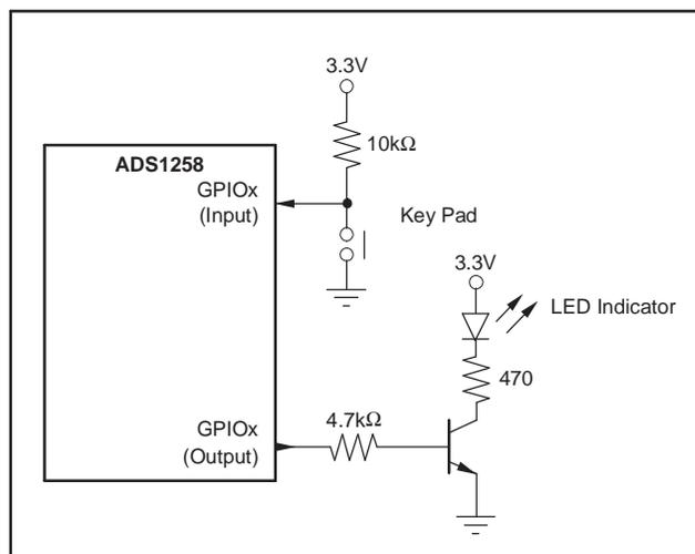
Figure 66. GPIO Connections
