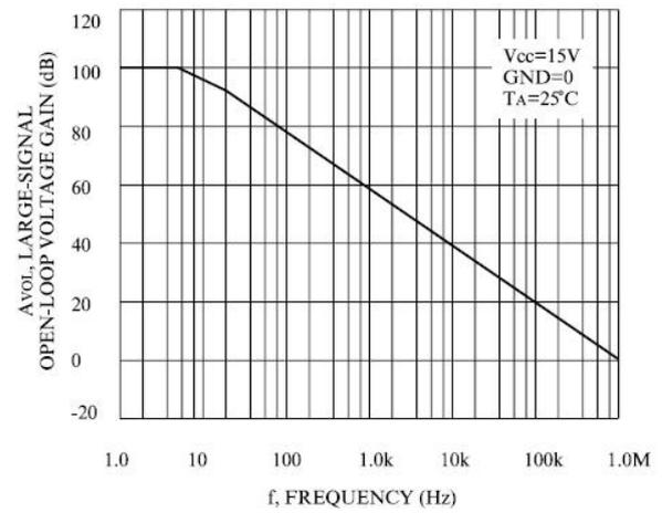
Figure 2. Open-Loop Frequency
