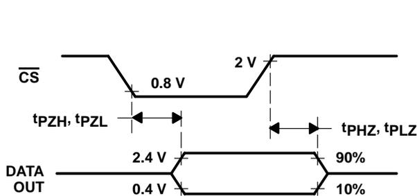
Figure 3. DATA OUT to Hi-Z Voltage Waveforms
