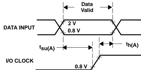
Figure 4. DATA INPUT and I/O CLOCK Voltage Waveforms
