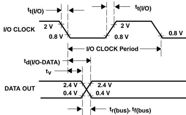
**Figure 6. I/O CLOCK and DATA OUT Voltage Waveforms**
