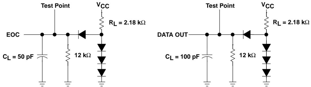
Figure 2. Load Circuits
