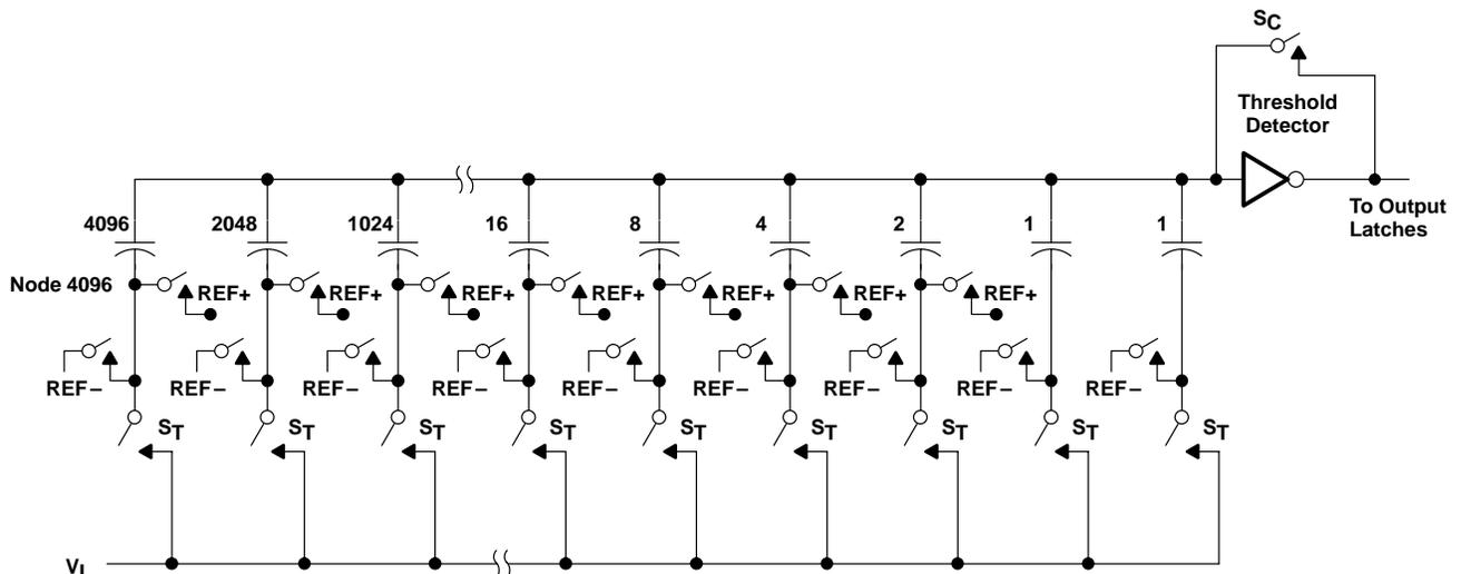
Figure 15. Simplified Model of the Successive-Approximation System
