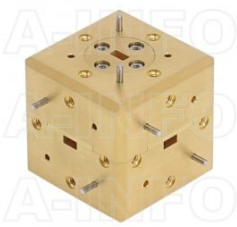
19WMT_Cu WR19 Waveguide Magic Tee 40-60GHz with Four Rectangular Waveguide Interfaces
