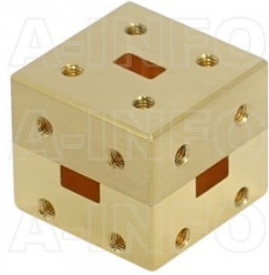
28WMT_Cu WR28 Waveguide Magic Tee 26.5-40GHz with Four Rectangular Waveguide Interfaces
