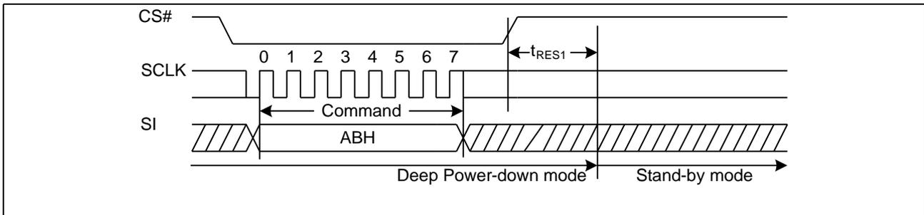
**Figure 25. Release Power-Down/Read Device ID Sequence Diagram**
