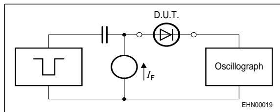
Pulse generator:  $t_p = 10\mu\text{s}$ ,  $D = 0.05$ ,  $t_r = 0.6\text{ns}$ ,
