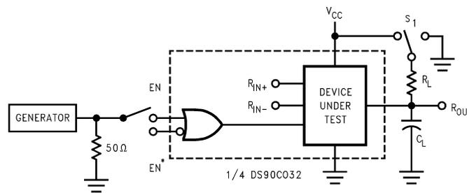
$C_L$  includes load and test jig capacitance.
