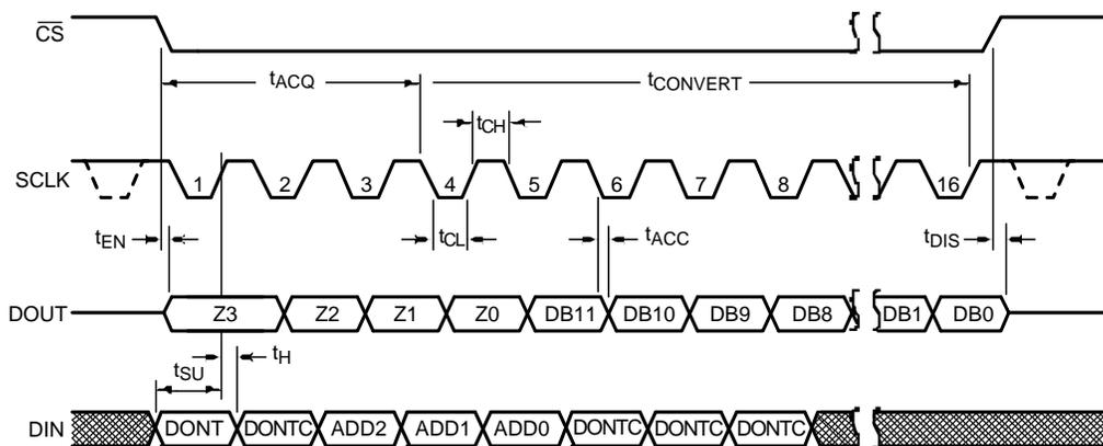
Figure 3. ADC122S021 Serial Timing Diagram
