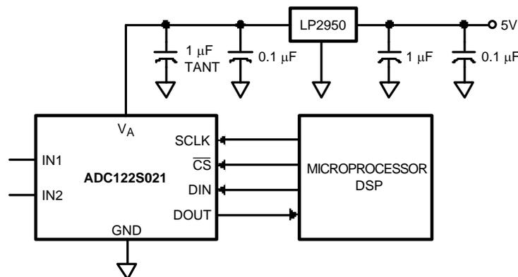
Figure 48. Typical Application Circuit
