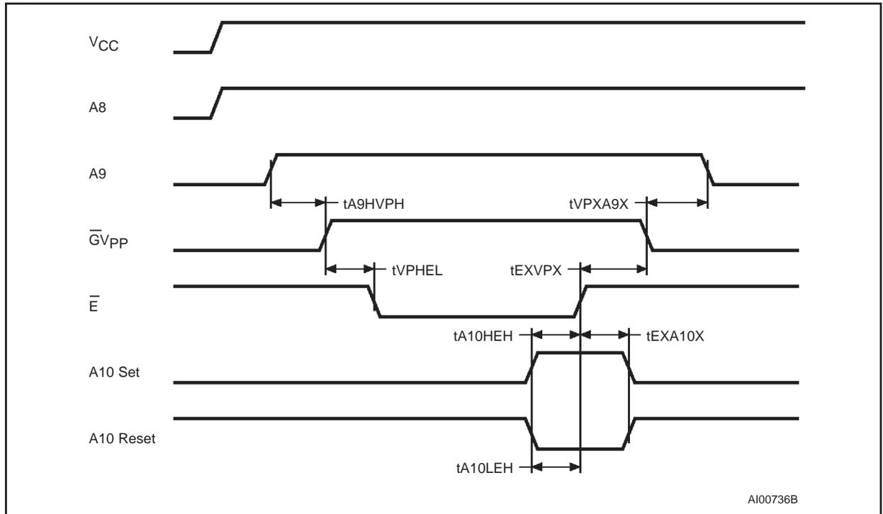
Note: A8 High level = 5V; A9 High level = 12V.
