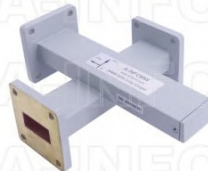
90WL+C-30_Cu WR90 Waveguide Cross Coupler WL+C-XX Type 8.2-12.4GHz 30dB Coupling with Three Rectangular Waveguide Interfaces
