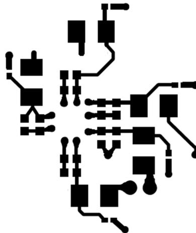
Figure 34. DS90C124 Example Layout of Power Decoupling from EVM
