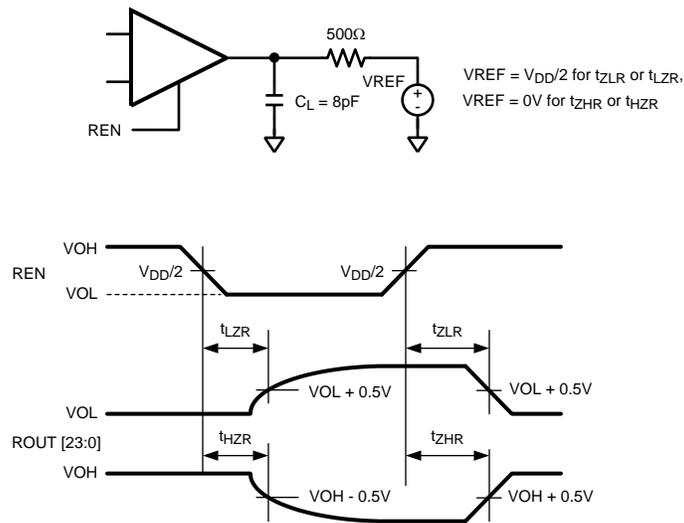
$C_L$  includes instrumentation and fixture capacitance within 6 cm of ROUT[23:0].
