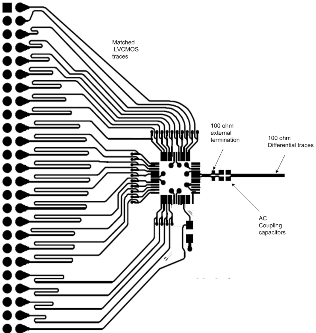
Figure 31. DS90C241 Layout Example from DS90C241 EVM
