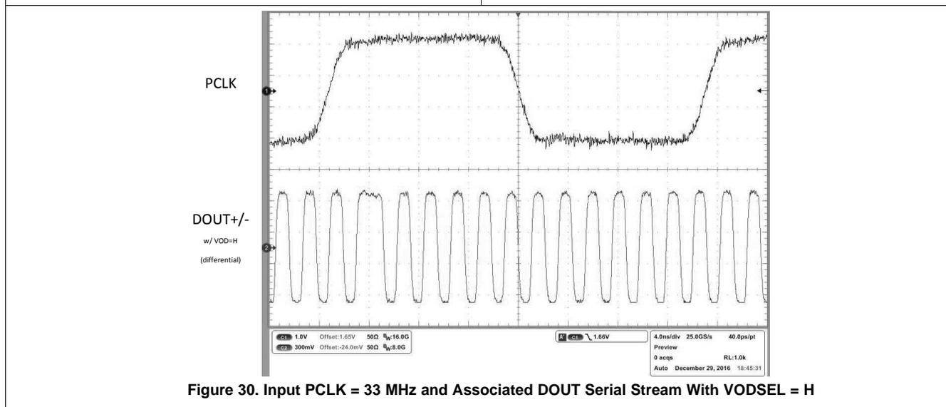
Figure 30. Input PCLK = 33 MHz and Associated DOUT Serial Stream With VODSEL = H
