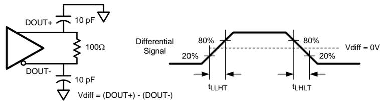
Figure 5. Serializer LVDS Output Load and Transition Times
