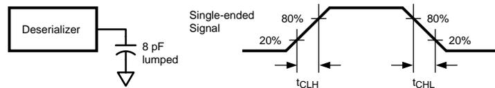
**Figure 13. Deserializer LVCMOS/LVTTL Output Load and Transition Times**
