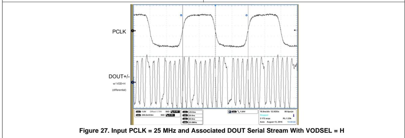
Figure 27. Input PCLK = 25 MHz and Associated DOUT Serial Stream With VODSEL = H
