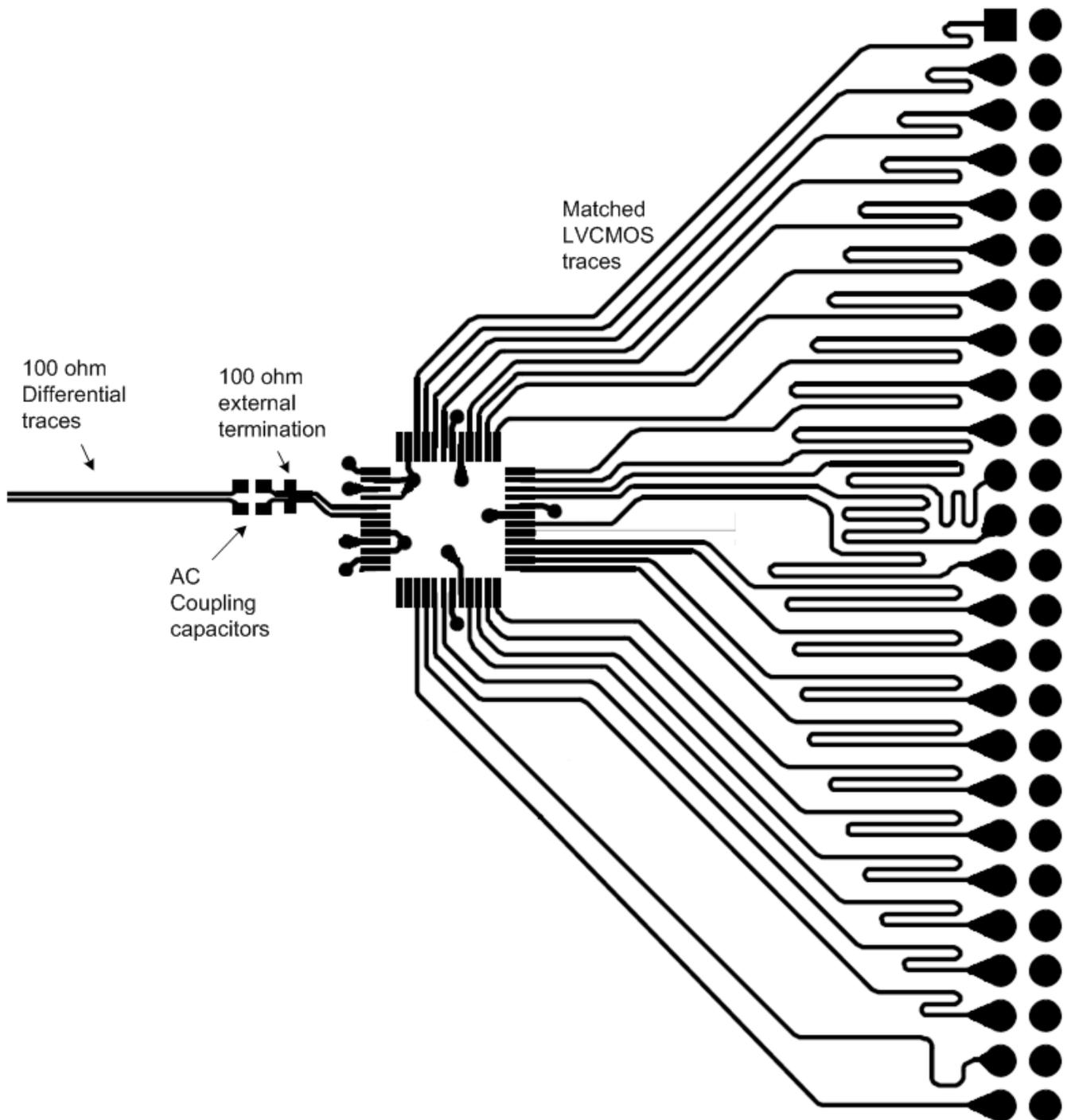
Figure 32. DS90C124 Layout Example from DS90C124 EVM
