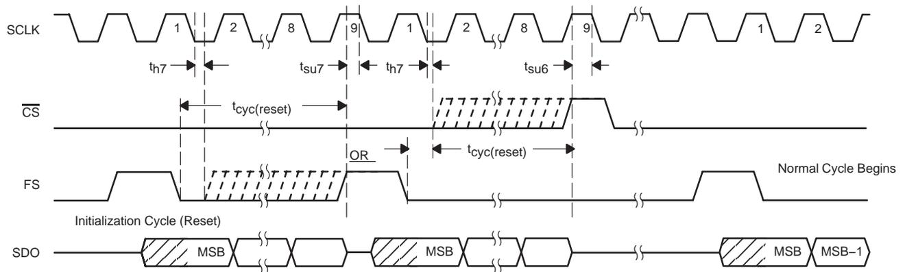
Figure 21. Critical Timing: Initialization Cycle (TLC3541 Only)
