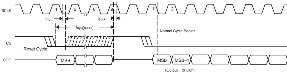
Figure 20. Critical Timing: Reset/Initialization Cycle (FS =1 for TLC3541)
