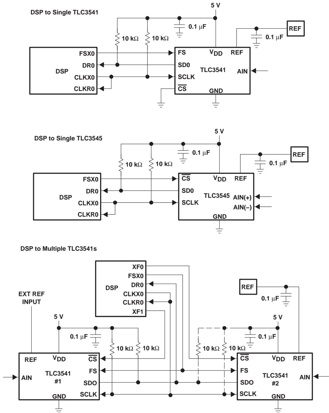
Figure 23. Typical ADC Interface to a TMS320 DSP
