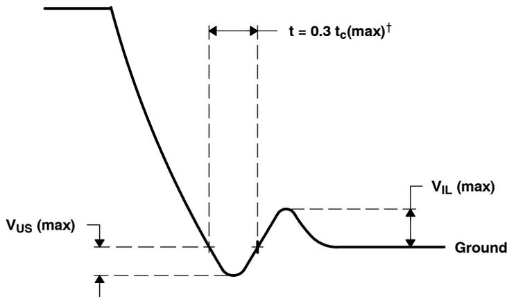
**Figure 19. AC Transient Specification Fall Time**
