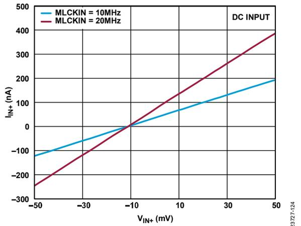
Figure 24.  $V_{IN+}$  Current ( $I_{IN+}$ ) vs.  $V_{IN+}$ , DC Input
