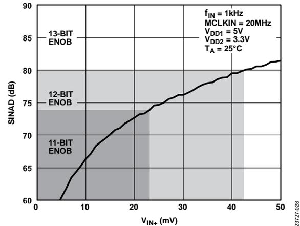
Figure 28. SINAD vs.  $V_{IN+}$  AC Input Signal Amplitude
