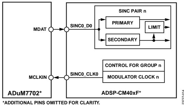
Figure 32. Interfacing the ADuM7702 to the ADSP-CM4xx
