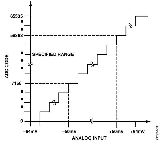
Figure 27. Filtered and Decimated 16-Bit Transfer Function
