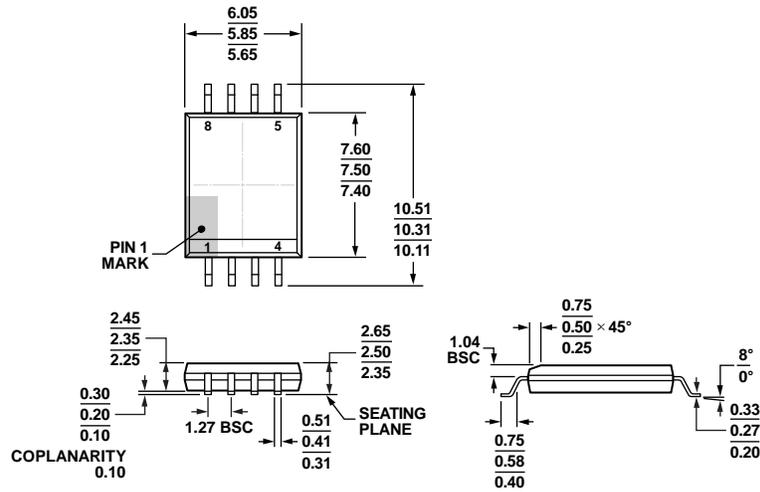
Figure 35. 8-Lead Standard Small Outline Package, with Increased Creepage [SOIC\_IC]
