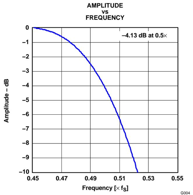
Figure 4. Transition-Band Characteristics
