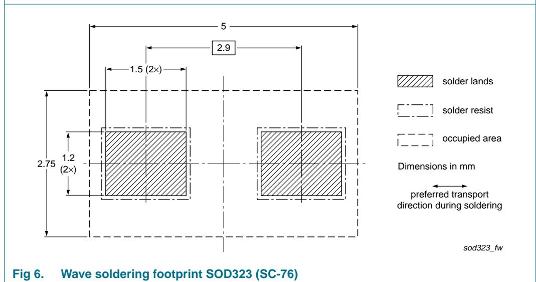
Fig 6. Wave soldering footprint SOD323 (SC-76)
