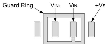
Figure 6. Example Guard Ring Layout for Non-Inverting Comparator
