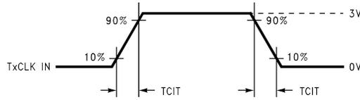
Figure 5. DS90C365A (Transmitter) Input Clock Transition Time
