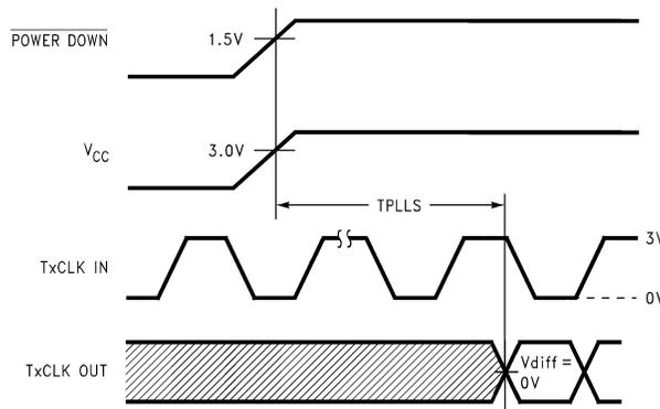
Figure 9. DS90C365A (Transmitter) Phase Lock Loop Set Time
