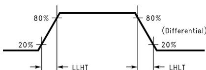
**Figure 4. DS90C365A (Transmitter) LVDS Transition Times**
