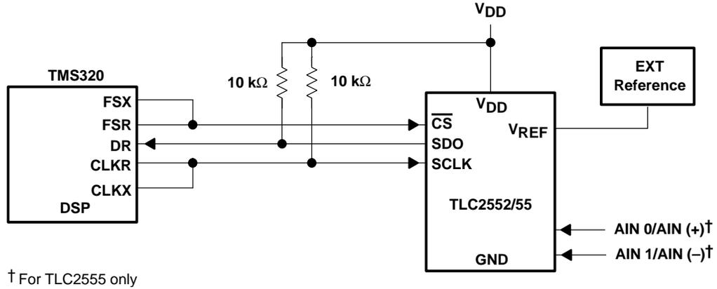
Figure 22. Typical TLC2552/55 Interface to a TMS320 DSP
