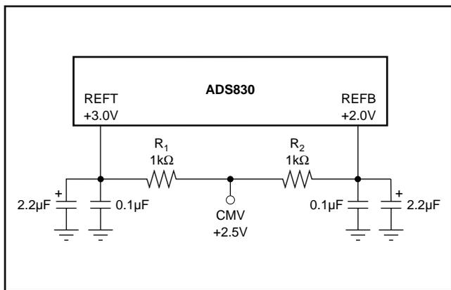
FIGURE 7. Alternative Circuit to Generate Common-Mode Voltage.
