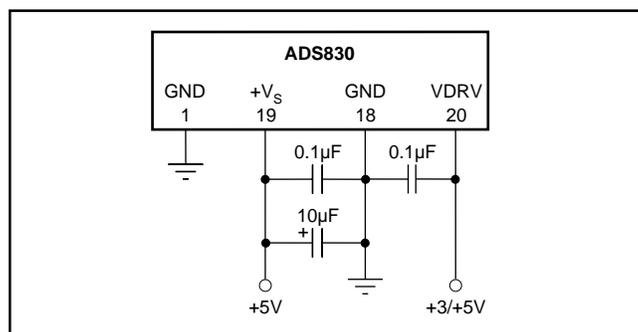
FIGURE 9. Recommended Bypassing for the Supply Pins.
