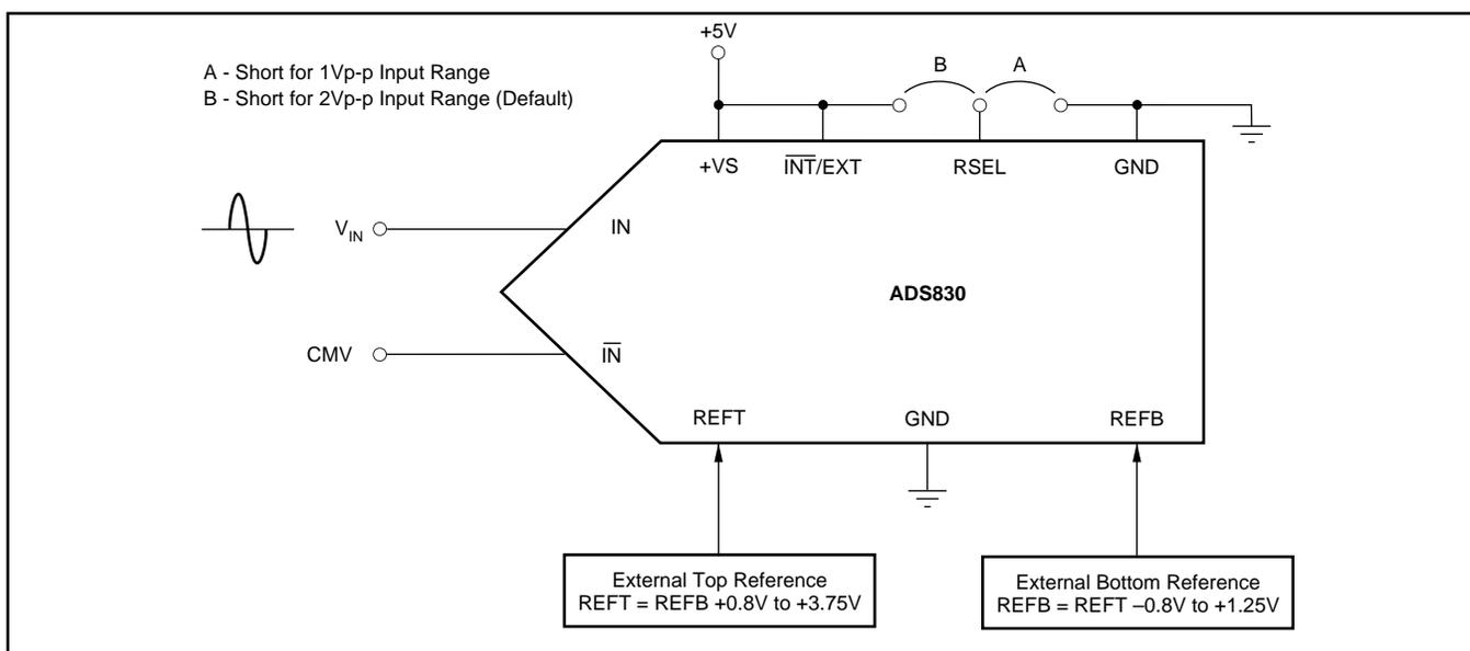
FIGURE 8. Configuration Example for External Reference Operation.
