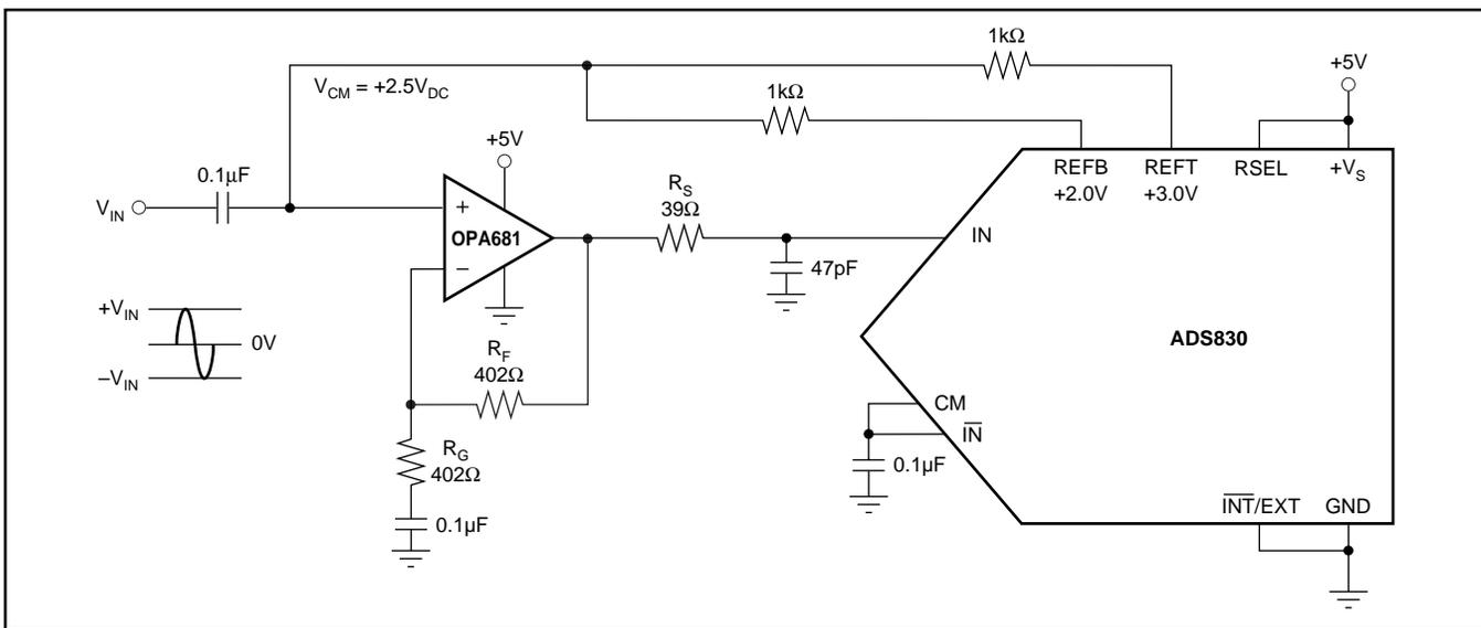
FIGURE 2. AC-Coupled Input Configuration for a 2Vp-p Full-Scale Range and a Common-Mode Voltage,  $V_{CM}$ , at +2.5V Derived from the Internal Top (REFT) and Bottom Reference (REFB). The OPA680 can be used in place of the OPA681 if a voltage feedback amplifier is preferred.
