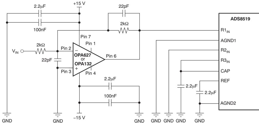
Figure 31. Typical Driving Circuitry (±10V, No Trim)
