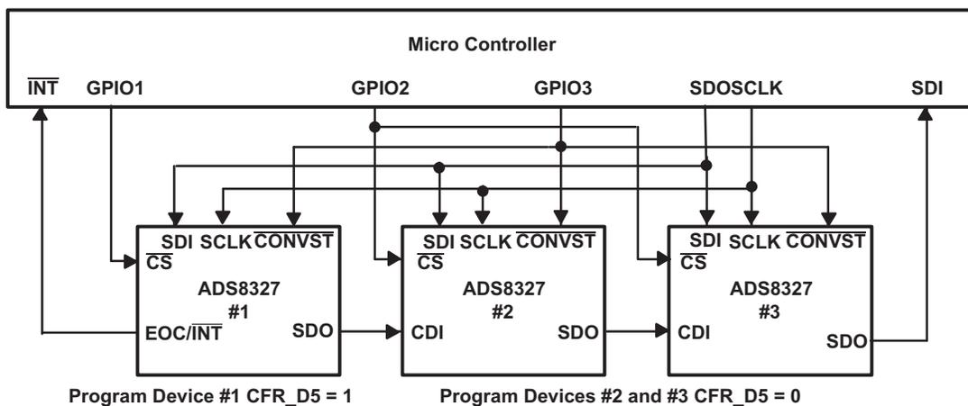
**Figure 59. Multiple Converters Connected Using Chain Mode**
