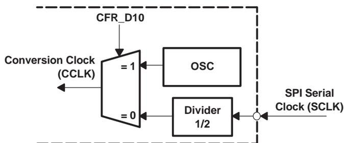
Figure 54. Converter Clock
