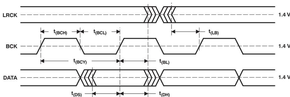
**Figure 22. Audio Interface Timing**
