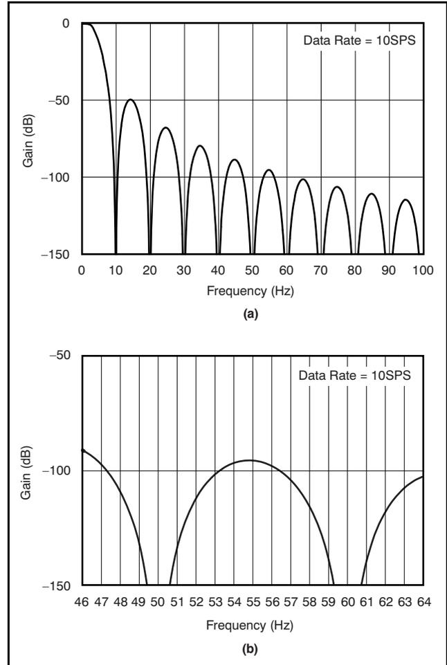
Figure 17. Nominal Frequency Response Out To 100Hz
