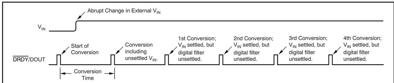
Figure 18. Settling Time in Continuous Conversion Mode
