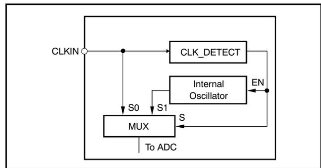
Figure 16. Equivalent Circuitry of the Clock Source
