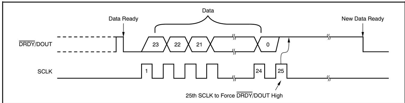
Figure 20. Data Retrieval with  $\overline{\text{DRDY}}/\text{DOUT}$  Forced High Afterwards
