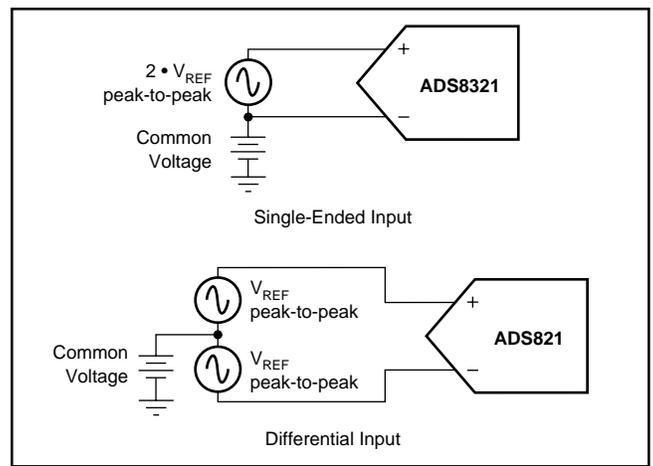
FIGURE 1. Methods of Driving the ADS8321—Single-Ended or Differential.
