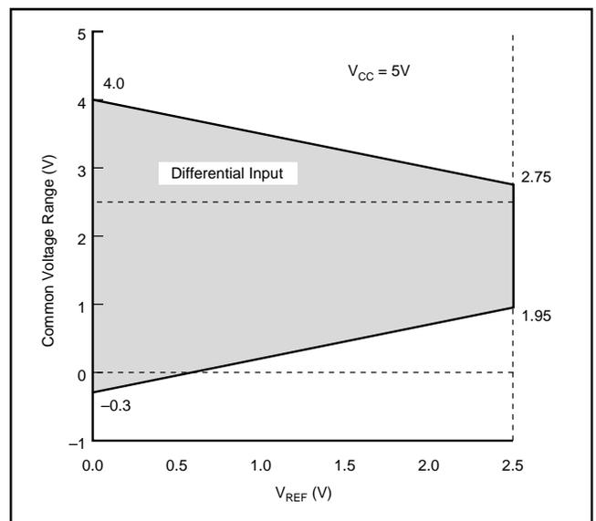
FIGURE 3. Differential Input—Common Voltage Range vs  $V_{REF}$ .
