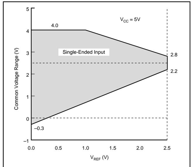
FIGURE 2. Single-Ended Input—Common Voltage Range vs  $V_{REF}$ .
