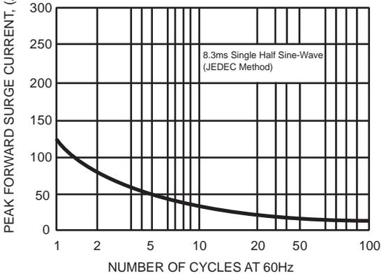
FIG. 2 - TYPICAL FORWARD CURRENT DERATING CURVE
