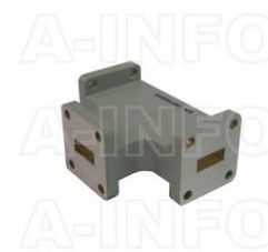
51WHT WR51 Waveguide H-Plane Tee 15-22GHz with Three Rectangular Waveguide Interfaces
