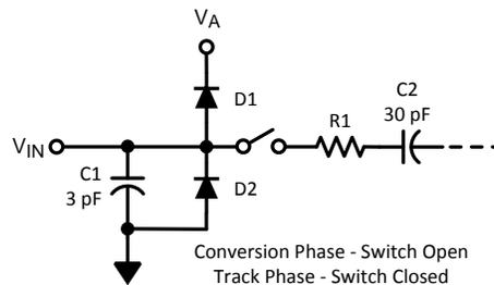
**Figure 52. Equivalent Input Circuit**
