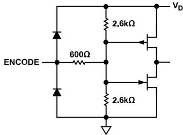
Figure 7. Encode Inputs
