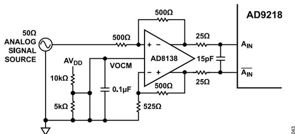
Figure 43. Using the AD8138 to Drive the AD9218
