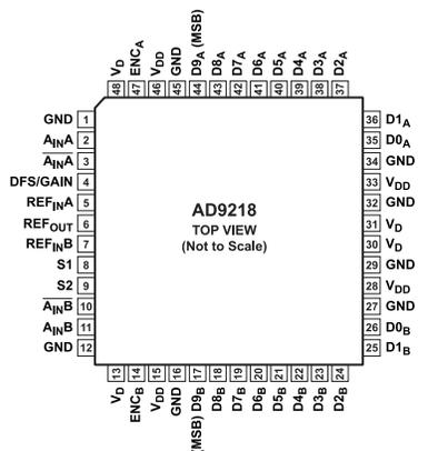
Figure 5. Pin Configuration
