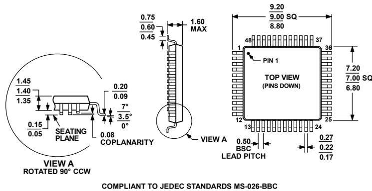
Figure 53. 48-Lead Low Profile Quad Flat Package [LQFP] (ST-48)
