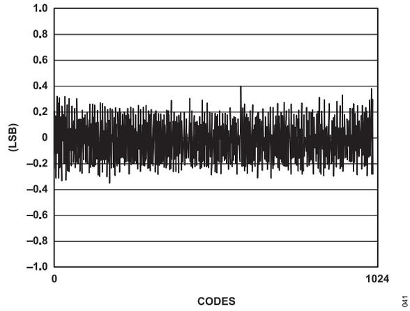
Figure 41. Typical DNL Plot, 10.3 MHz  $A_{IN}$  @ 80 MSPS
