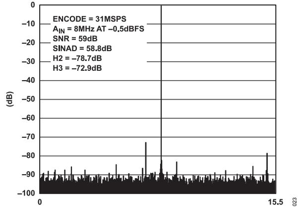
Figure 23. FFT: FS = 31 MSPS,  $A_{IN}$  = 8 MHz @ -0.5 dBFS, Differential, with AD8138 Driving ADC Inputs, 1 V p-p Input Range
