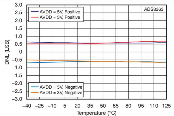
Figure 8. Differential Nonlinearity vs Temperature
