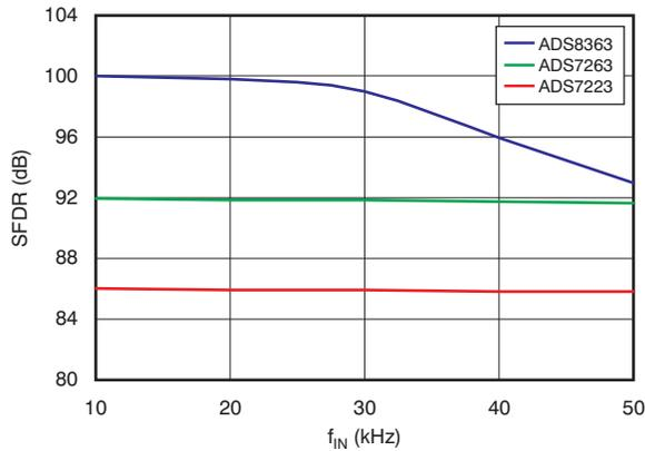
Figure 21. Spurious-Free Dynamic Range vs Input Signal Frequency
