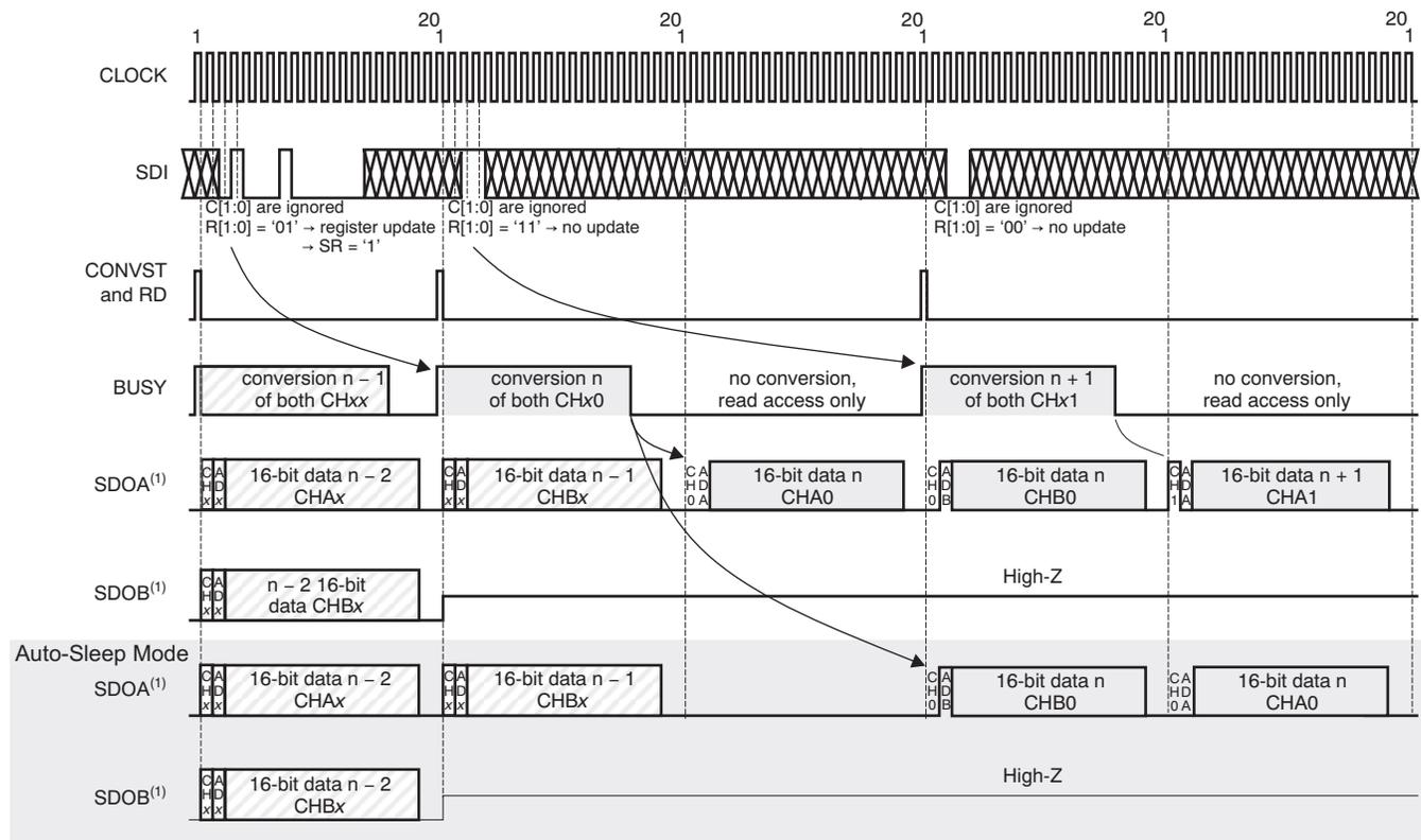
(1) The ADS7263 and ADS7223 output data with the MSB located as the ADS8363 and the last 2 or 4 bits are '0'.
