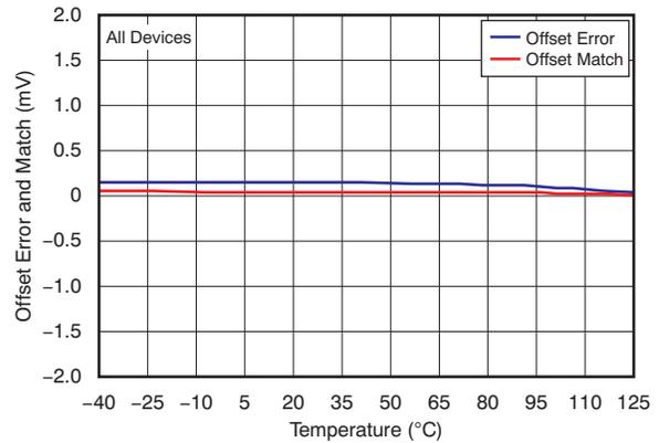
**Figure 10. Offset Error and Offset Match vs Temperature**
