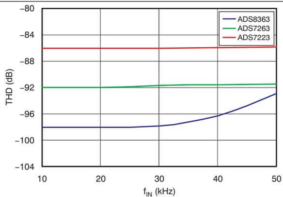
Figure 19. Total Harmonic Distortion vs Input Signal Frequency
