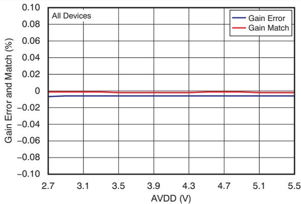
**Figure 11. Gain Error and Gain Match vs Analog Supply Voltage**
