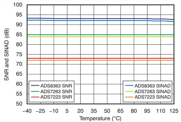
Figure 18. Signal-to-Noise Ratio and Signal-to-Noise + Distortion vs Temperature
