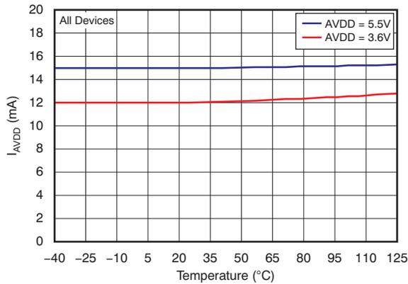
Figure 23. Analog Supply Current vs Temperature
