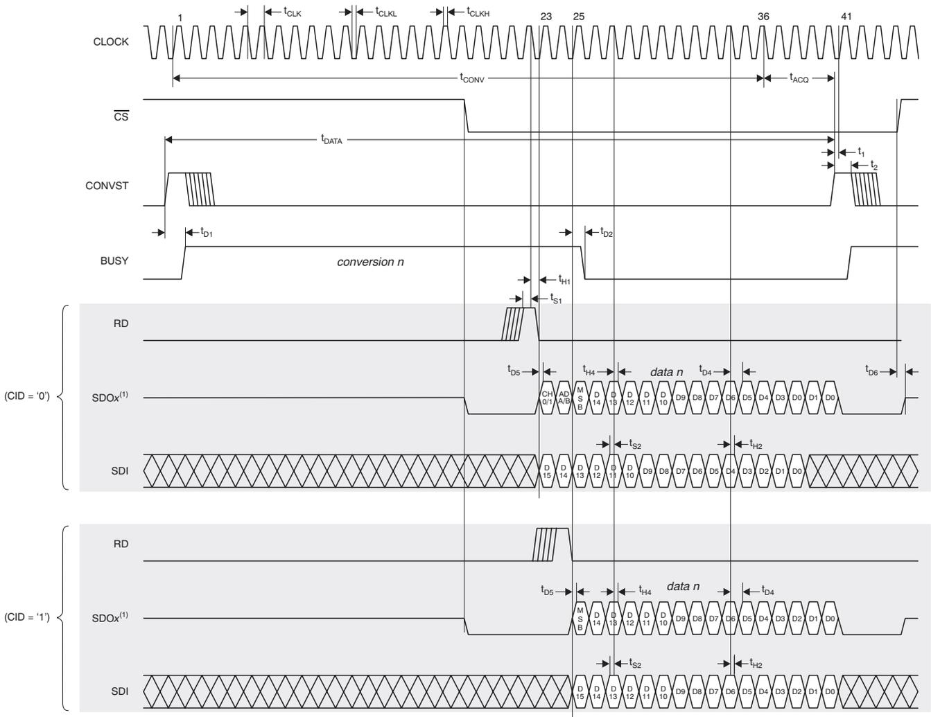
(2) The ADS7263 and ADS7223 output data with the MSB located as the ADS8363 and the last 2 or 4 bits are '0'.
