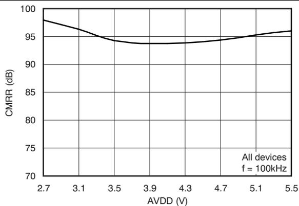
**Figure 13. Common-Mode Rejection Ratio vs Analog Supply Voltage**
