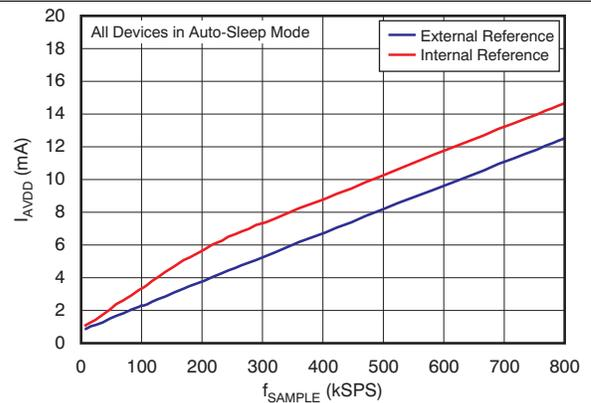
Figure 26. Analog Supply Current vs Data Rate (Auto-Sleep Mode)
