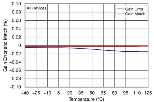
**Figure 12. Gain Error and Gain Match vs Temperature**
