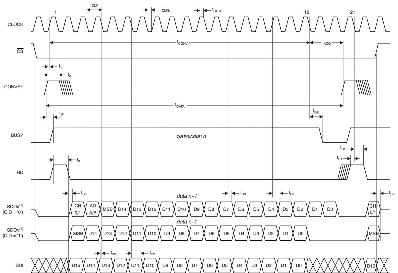
(1) The ADS7263 and ADS7223 output data with the MSB located as the ADS8363 and the last 2 or 4 bits are '0'.
