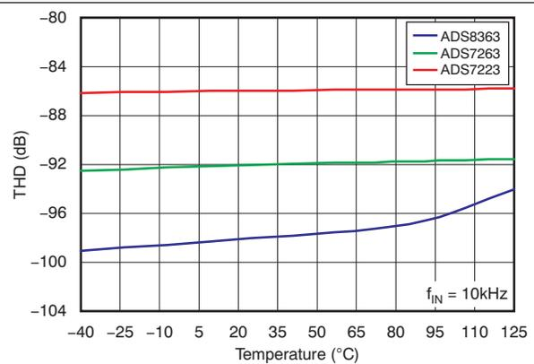
Figure 20. Total Harmonic Distortion vs Temperature
