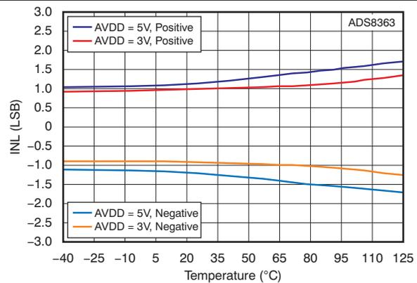
Figure 7. Integral Nonlinearity vs Temperature
