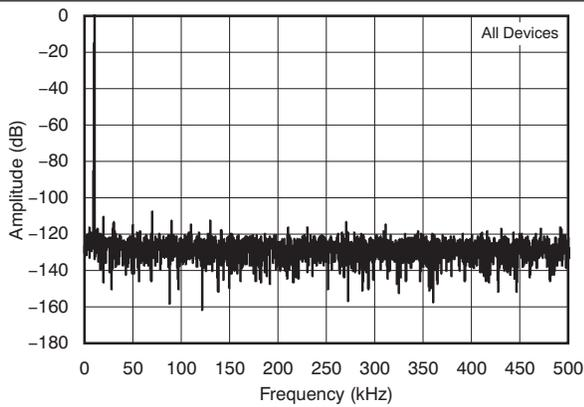
Figure 15. Frequency Spectrum (4096 Point FFT;  $f_{IN} = 10\text{ kHz}$ )
