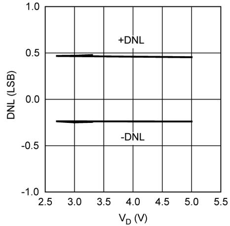
Figure 13. DNL vs  $V_D$  With  $V_A = 5 \text{ V}$
