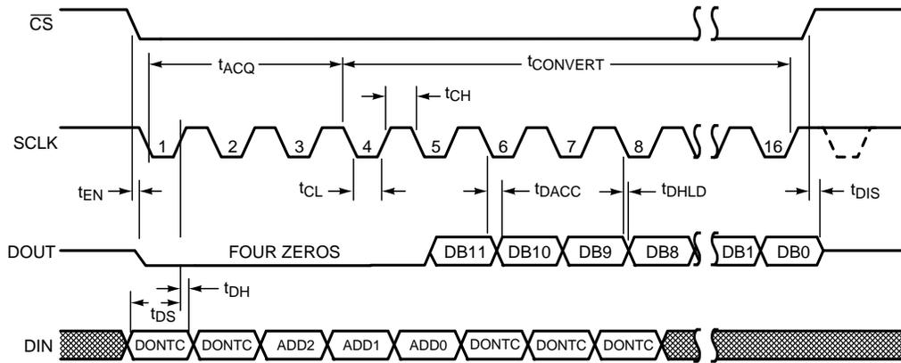
**Figure 2. ADC128S022 Serial Timing Diagram**
