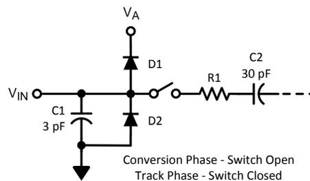
**Figure 37. Equivalent Input Circuit**
