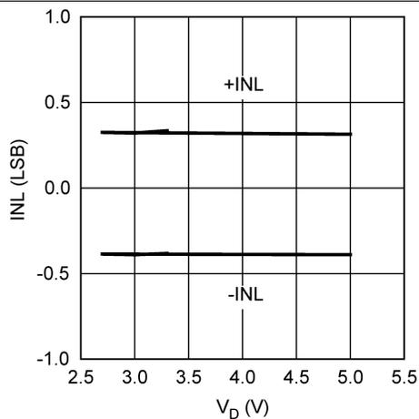
Figure 14. INL vs  $V_D$  With  $V_A = 5 \text{ V}$
