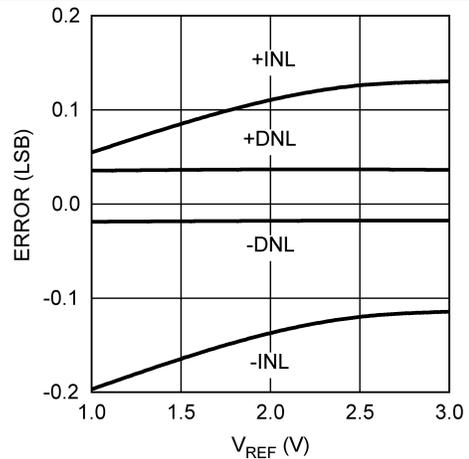
Figure 7. INL/DNL vs  $V_{REFIN}$  at  $V_A = 3$  V
