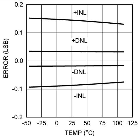
Figure 14. INL/DNL vs Temperature at  $V_A = 5$  V
