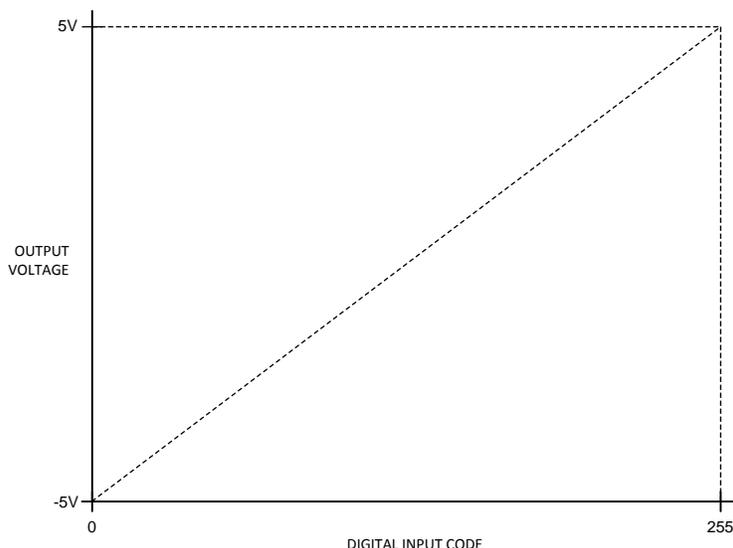
**Figure 36. Bipolar Input / Output Transfer Characteristic**
