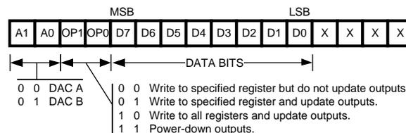
**Figure 30. Input Register Contents**
