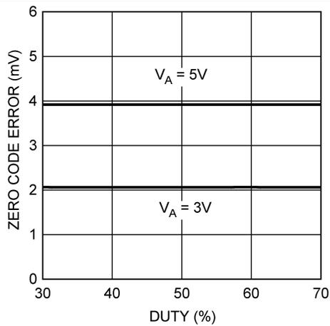
Figure 18. Zero Code Error vs Clock Duty Cycle
