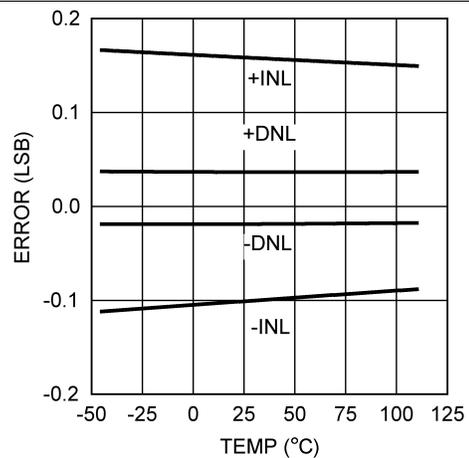
**Figure 13. INL/DNL vs Temperature at  $V_A = 3$  V**
