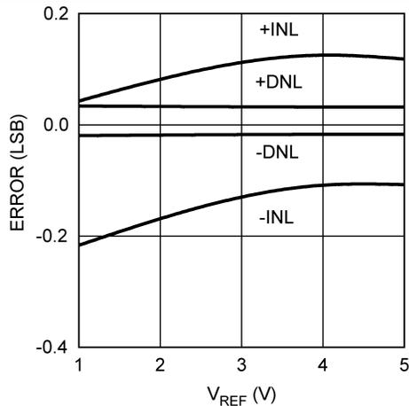
**Figure 8. INL/DNL vs  $V_{REFIN}$  at  $V_A = 5$  V**
