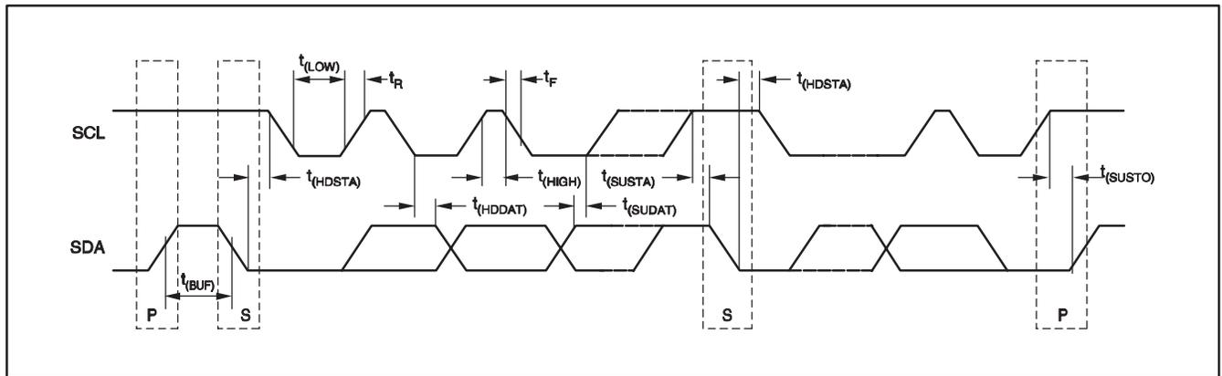
**Figure 1. I<sup>2</sup>C Timing Diagram**
