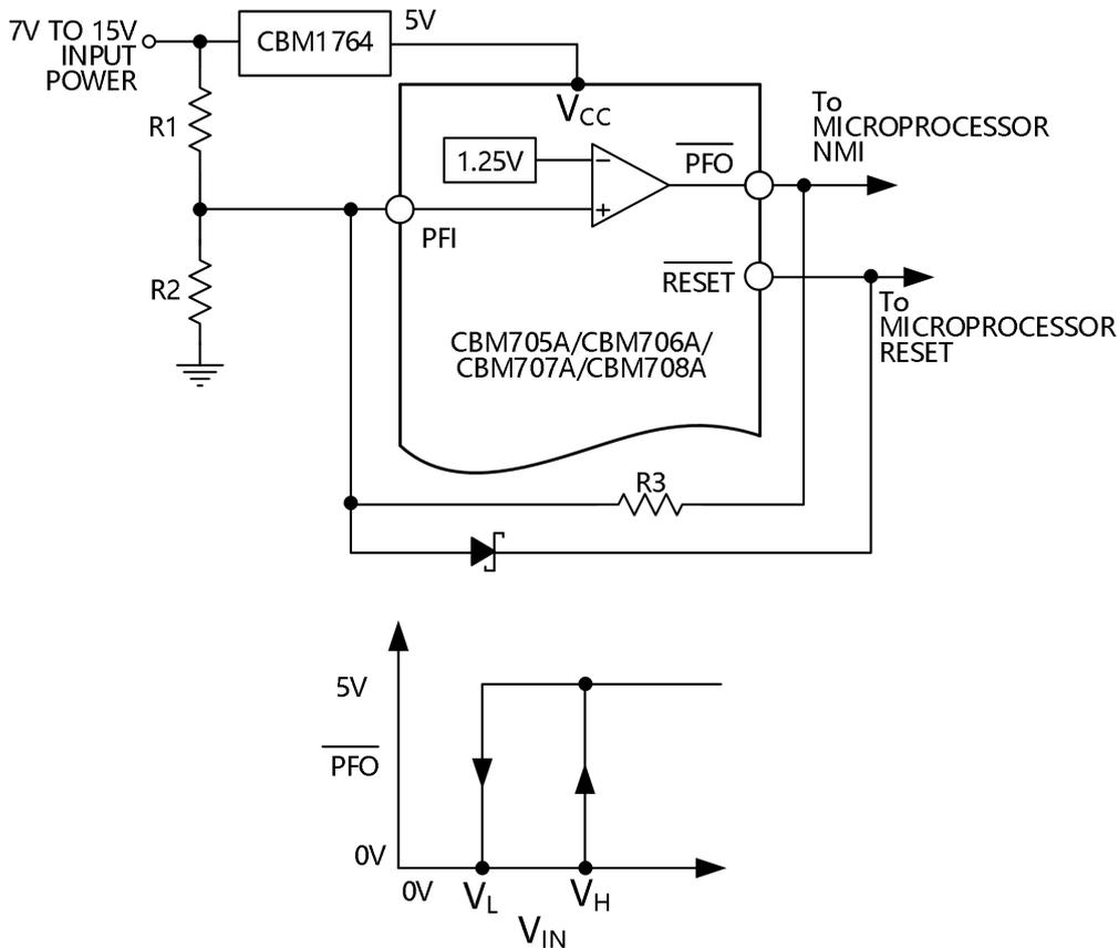
Figure 16. Adding Hysteresis to the Power Fail Comparator
