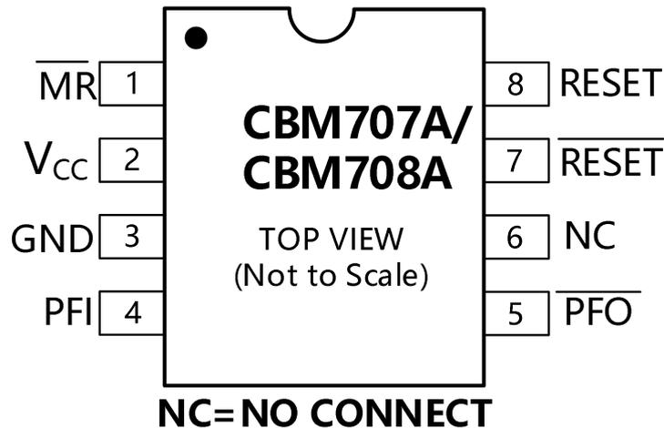
Figure 4. CBM707A/CBM708A PDIP/SOIC
