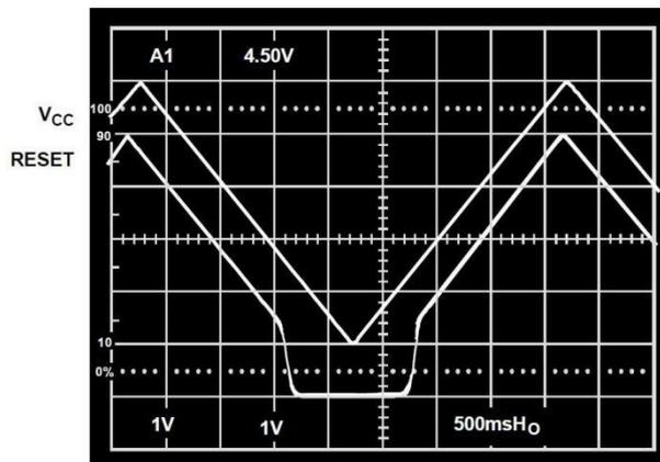
Figure 7. CBM707/CBM708 RESET Output vs. Supply Voltage
