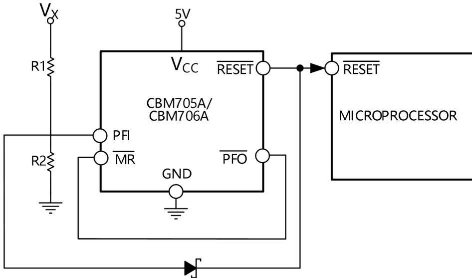
Figure 20. Monitoring 5 V and an Additional Supply, VX
