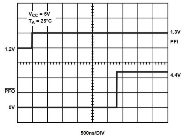
Figure 9. PFI Comparator Deassertion Voltage Response Time
