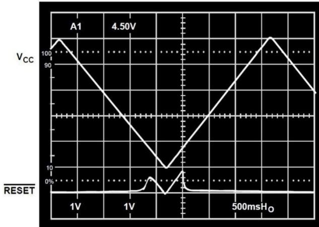
Figure 6. RESET Output Voltage vs. Supply Voltage
