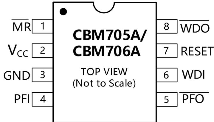
Figure 3. CBM705A/CBM706A PDIP/SOIC
