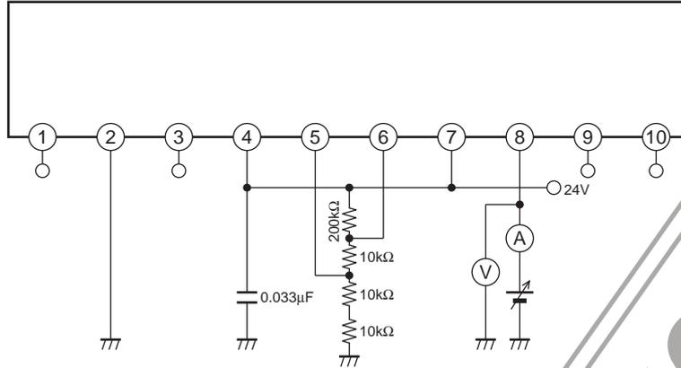
Read the reading on voltmeter (V) when ammeter (A) reads 20mA is Fig.3
