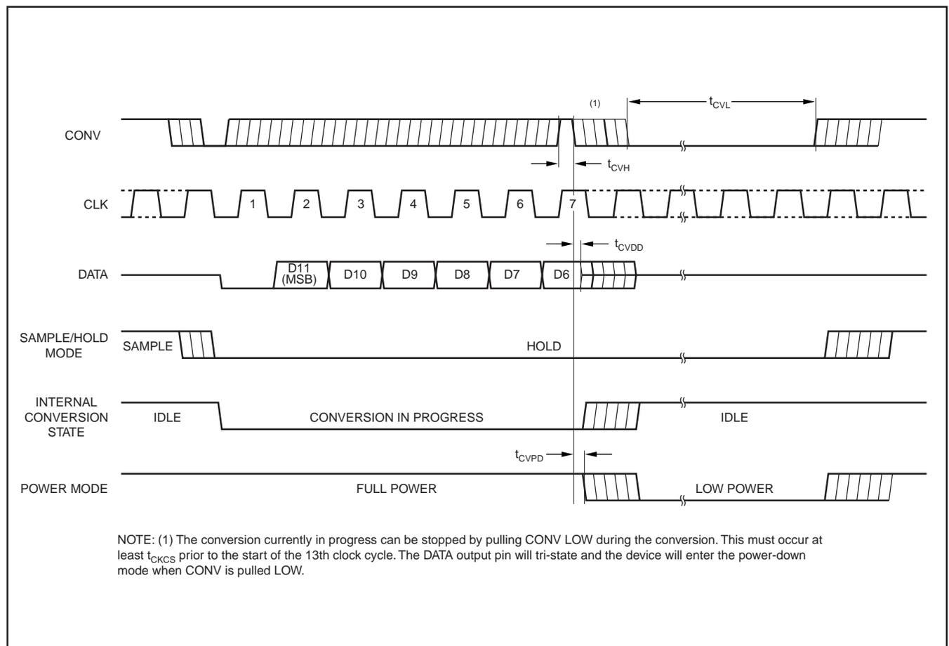
FIGURE 6. Short-Cycle Timing.
