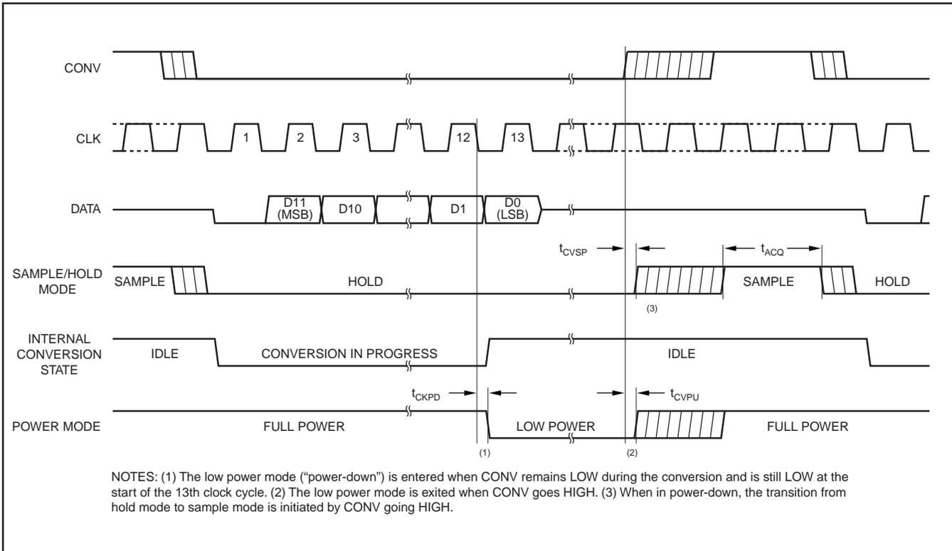
FIGURE 4. Power-Down Timing.
