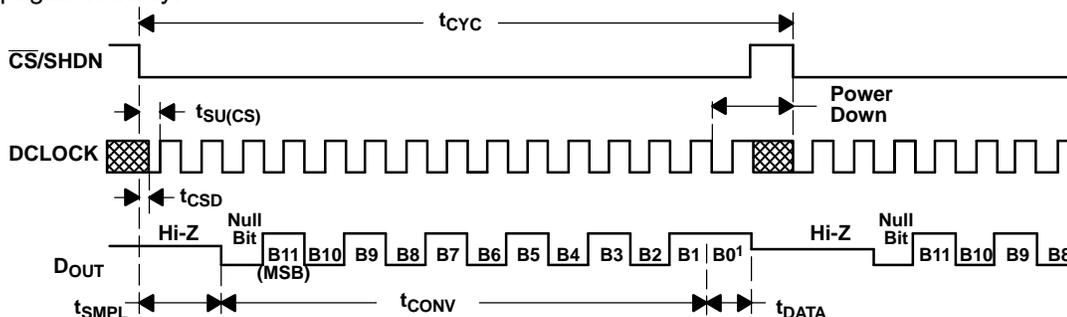
After completing the data transfer, if further clocks are applied with  $\overline{CS}$  LOW, the A/D outputs LSB-First data then followed with zeroes indefinitely.
