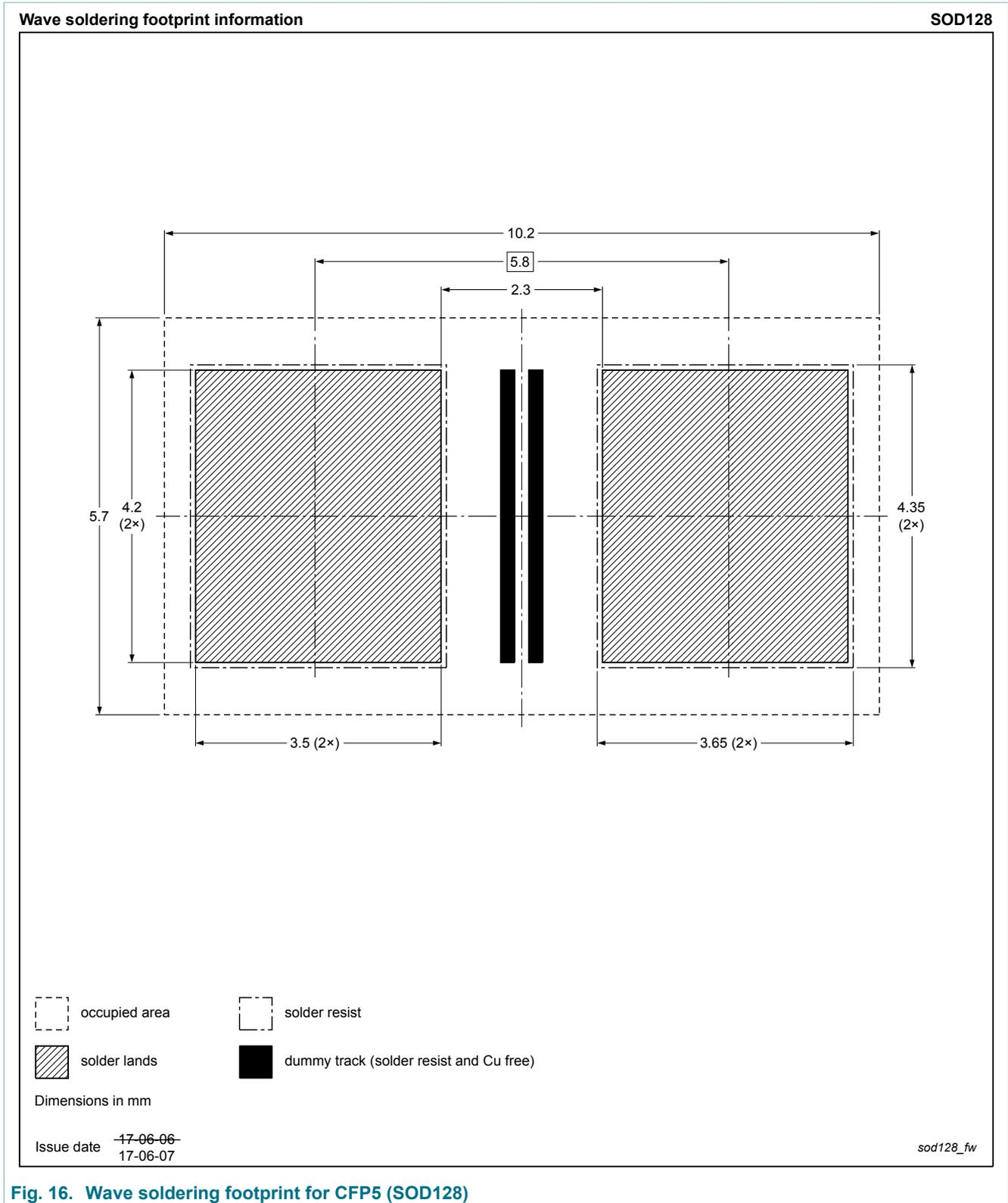
**Fig. 16. Wave soldering footprint for CFP5 (SOD128)**
