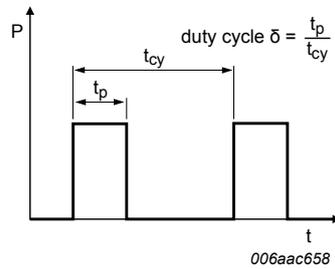
Fig. 13. Duty cycle definition
