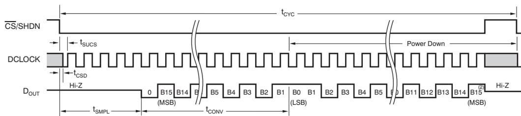
NOTE: (2) After completing the data transfer, if further clocks are applied with CS low, the A/D converter will output zeroes indefinitely.
