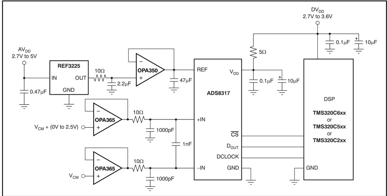
Figure 45. Example of a Basic Data Acquisition System
