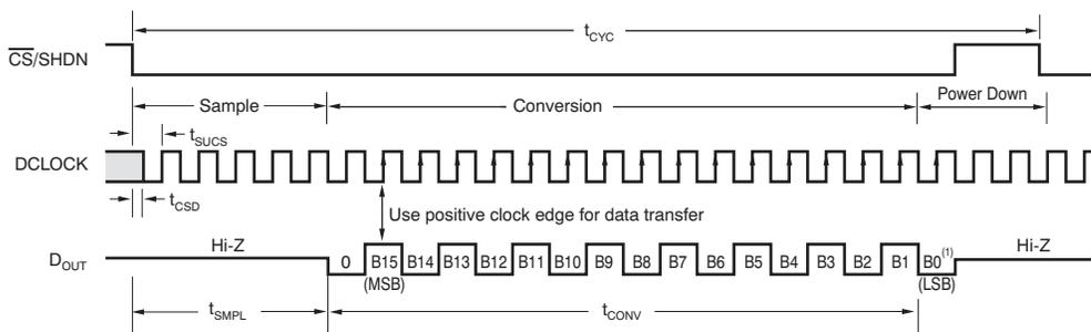
NOTE: (1) A minimum of 22 clock cycles are required for 16-bit conversion; 24 clock cycles are shown. If CS remains low at the end of conversion, a new data stream is shifted out with LSB-first data followed by zeroes indefinitely.
