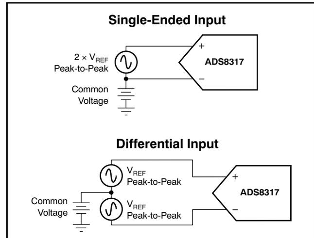
**Figure 37. Methods of Driving the ADS8317—Single-Ended or Differential**
