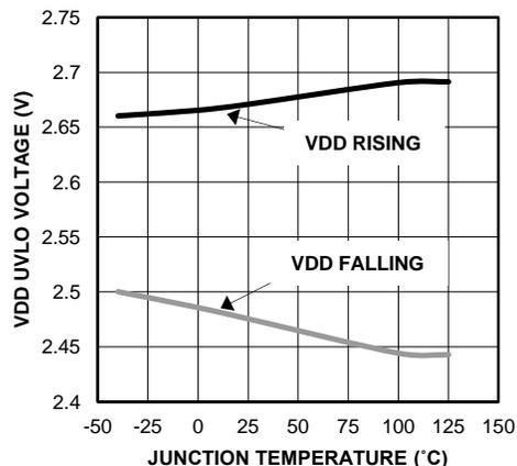
Figure 7. UVLO Thresholds
