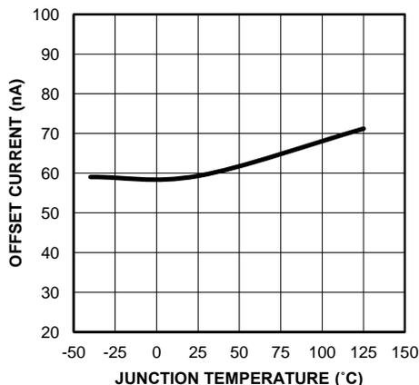
Figure 6. IDAC\_OUT Offset Current
