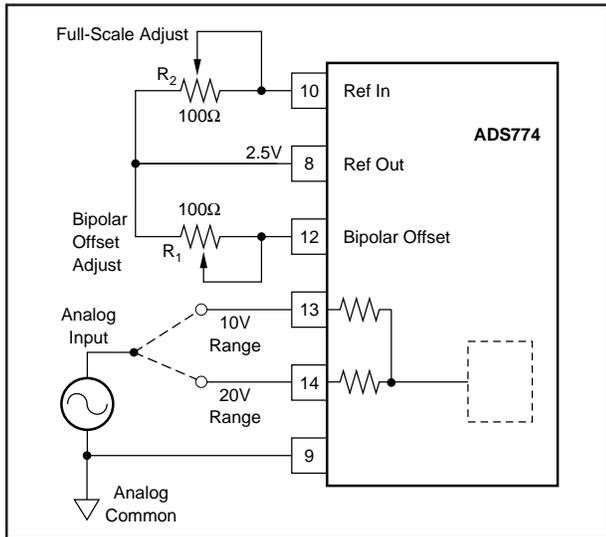
FIGURE 11. Bipolar Configuration.
