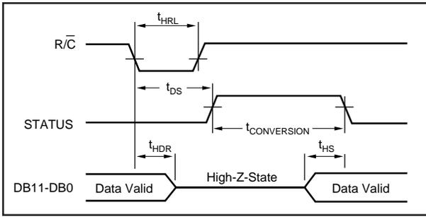
FIGURE 3. R/C Pulse Low—Outputs Enabled After Conversion.
