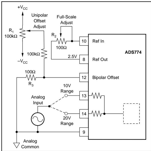
FIGURE 10. Unipolar Configuration.
