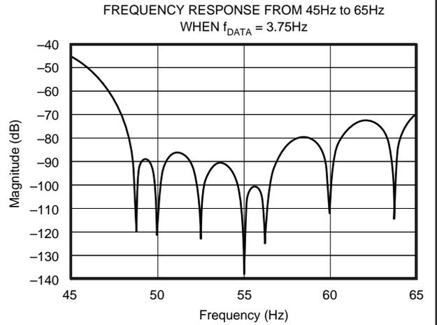
$f_{OSC} = 2.4576\text{MHz}$ , SPEED = 0 or  $f_{OSC} = 4.9152\text{MHz}$ , SPEED = 1
