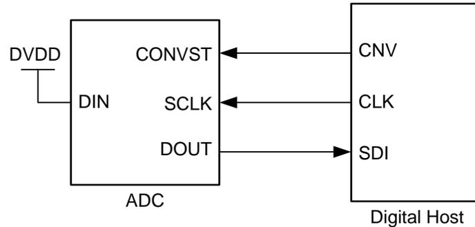
Figure 43. Connection Diagram: 3-Wire  $\overline{CS}$  Mode (DIN = 1)
