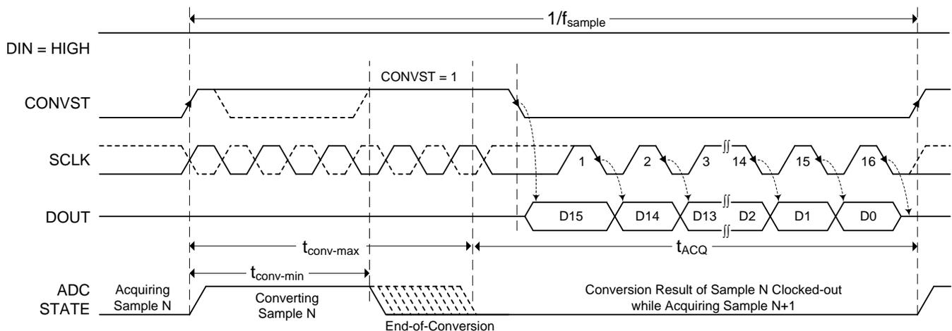
Figure 44. Interface Timing Diagram: 3-Wire  $\overline{CS}$  Mode (DIN = 1)
