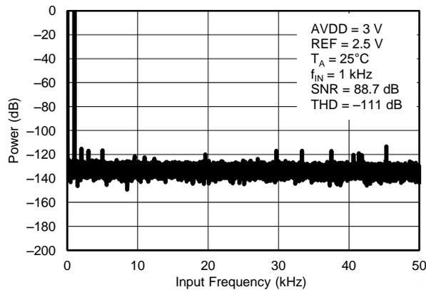
**Figure 16. TYPICAL FFT ( $V_{REF} = 2.5\text{ V}$ )**
