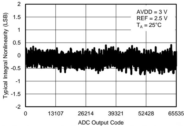
Figure 6. TYPICAL INL ( $V_{REF} = 2.5\text{ V}$ )
