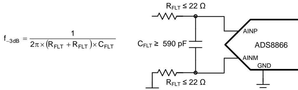
**Figure 56. Antialiasing Filter**
