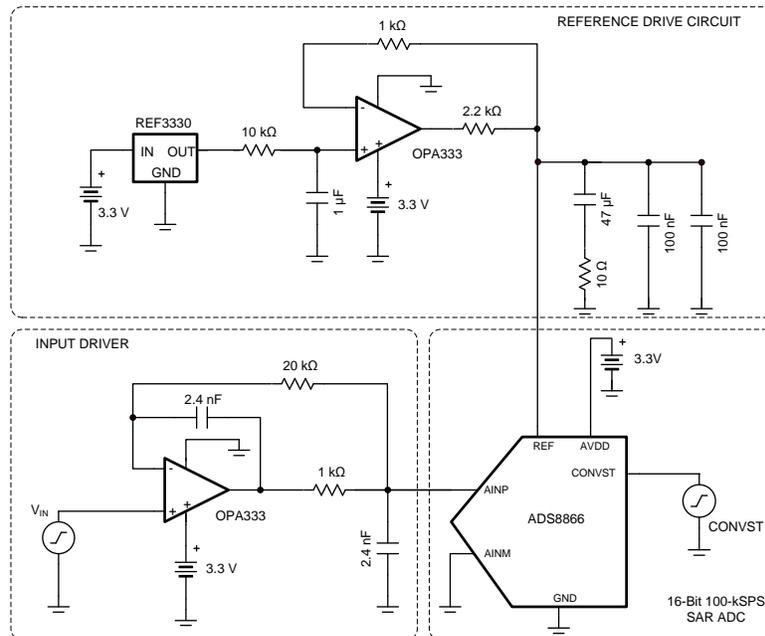
Figure 59. Ultralow-Power DAQ Circuit at 10 kSPS
