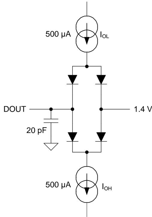
**Figure 4. Load Circuit for Digital Interface Timing**
