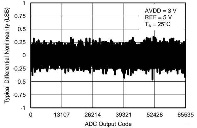
Figure 9. TYPICAL DNL ( $V_{REF} = 5\text{ V}$ )
