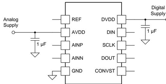
**Figure 51. Supply Decoupling**
