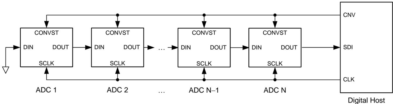
Figure 49. Connection Diagram: Daisy-Chain Mode (DIN = 0)
