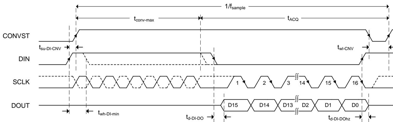
Figure 2. 4-Wire Operation: DIN Functions as Chip Select
