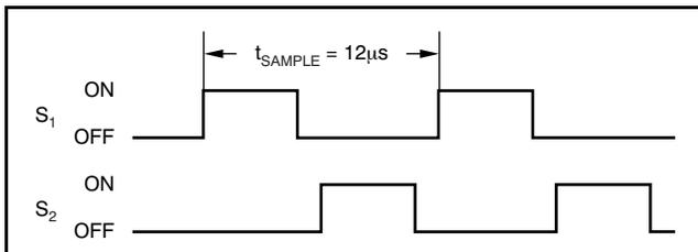
Figure 21.  $S_1$  and  $S_2$  Switch Timing for Figure 20
