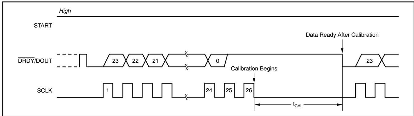
Figure 30. Self-Calibration Timing
