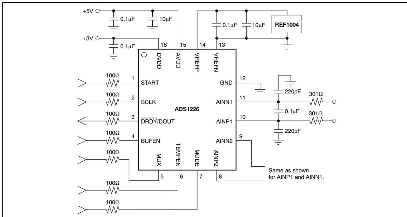
Figure 31. Basic Connections
