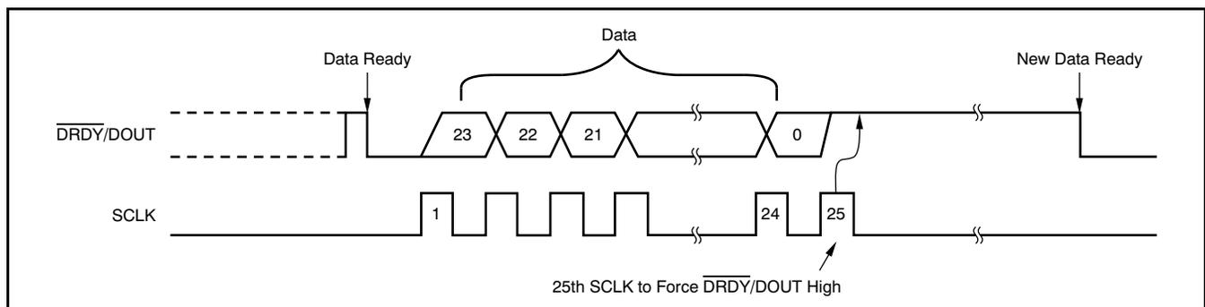
Figure 29. Data Retrieval with  $\overline{\text{DRDY}}/\text{DOUT}$  Forced High Afterwards
