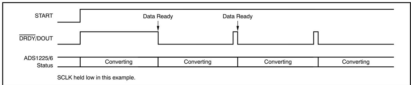
**Figure 27. Conversion with the START Pin High**
