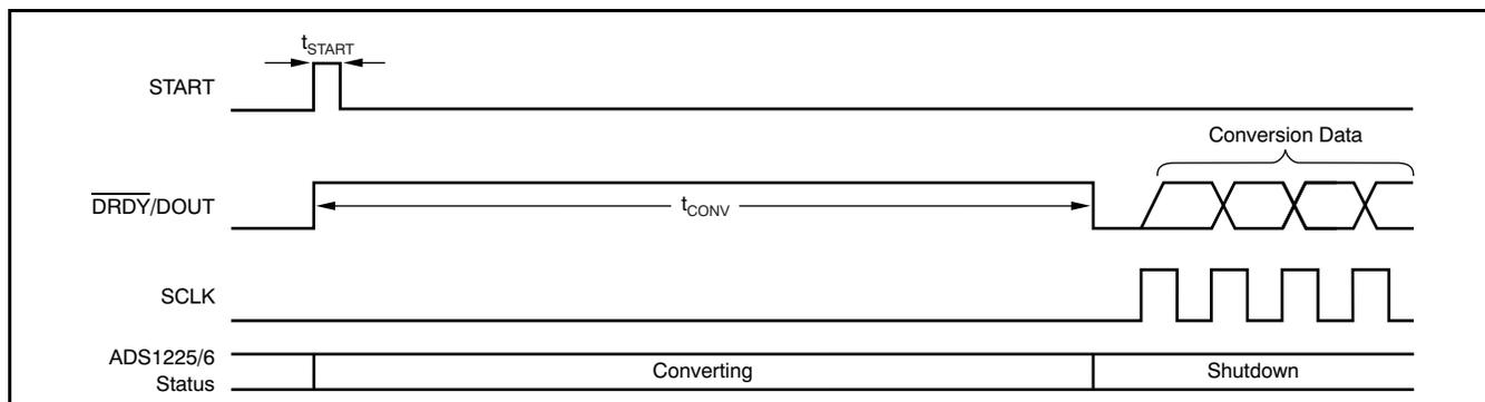
**Figure 26. Controlling Conversion with the START Pin**
