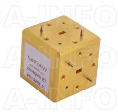
19WET_Cu WR19 Waveguide E-Plane Tee 40-60GHz with Three Rectangular Waveguide Interfaces
