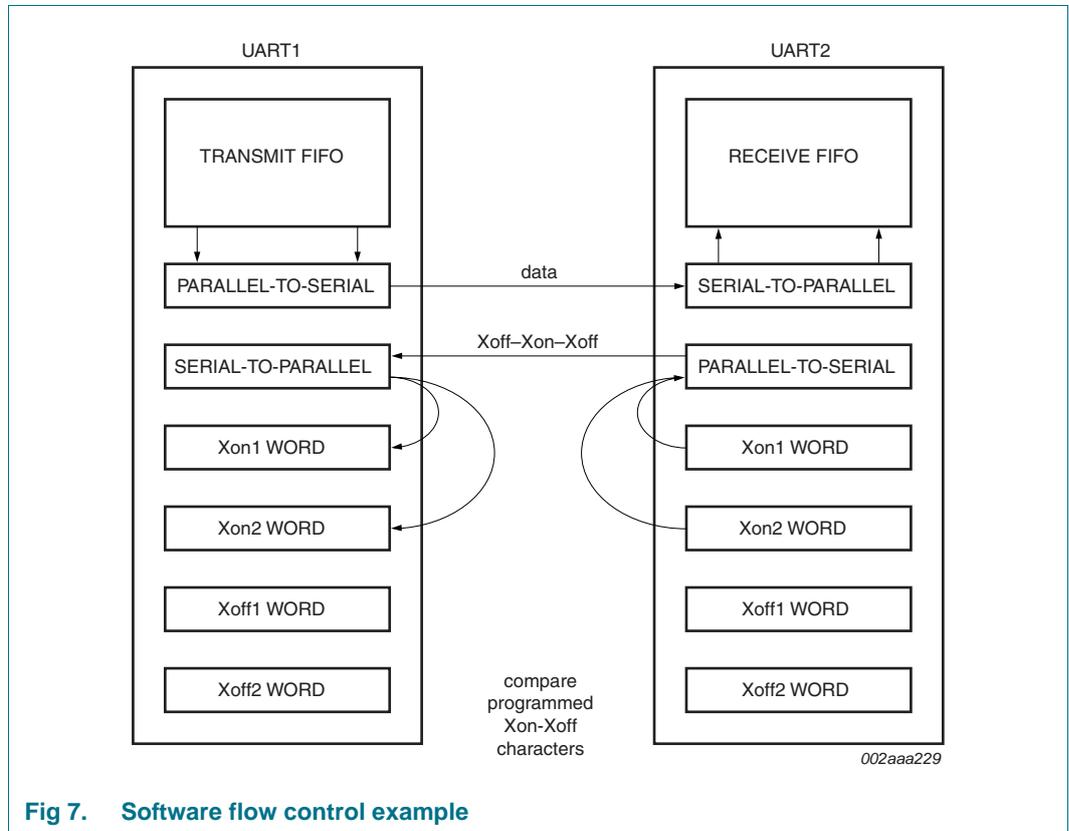
Fig 7. Software flow control example
