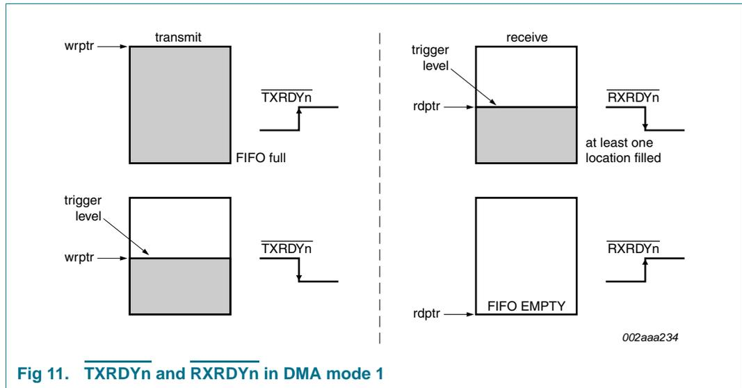
Fig 11. TXRDYn and RXRDYn in DMA mode 1
