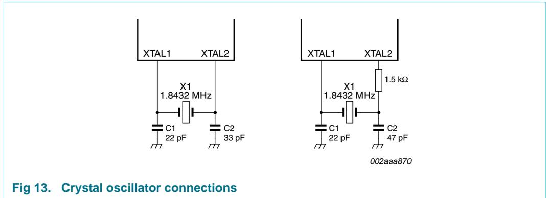
Fig 13. Crystal oscillator connections
