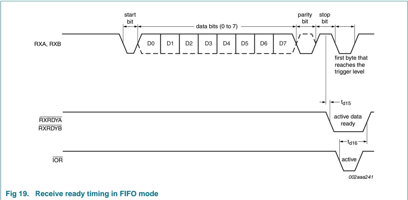
Fig 19. Receive ready timing in FIFO mode
