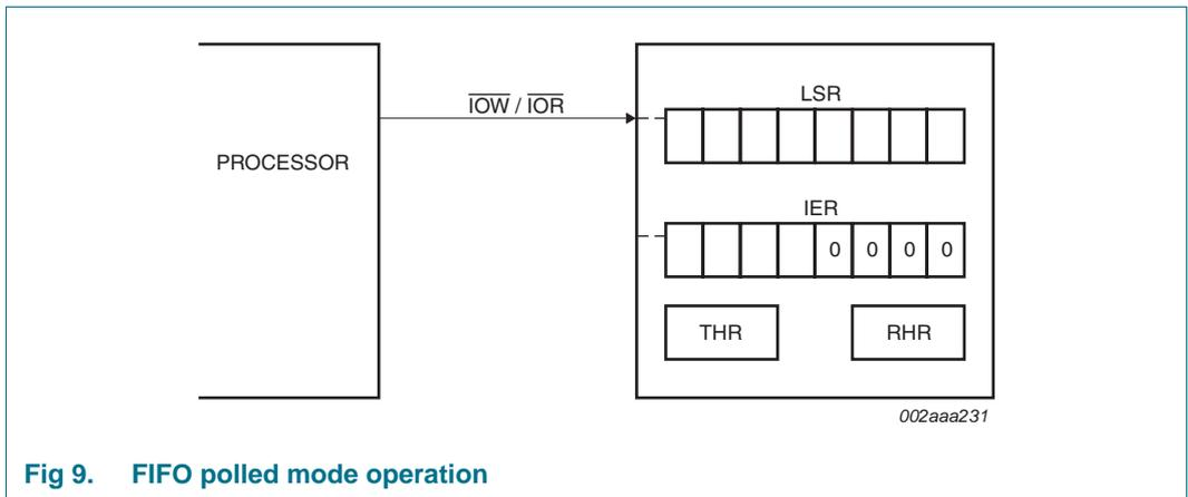
**Fig 9. FIFO polled mode operation**
