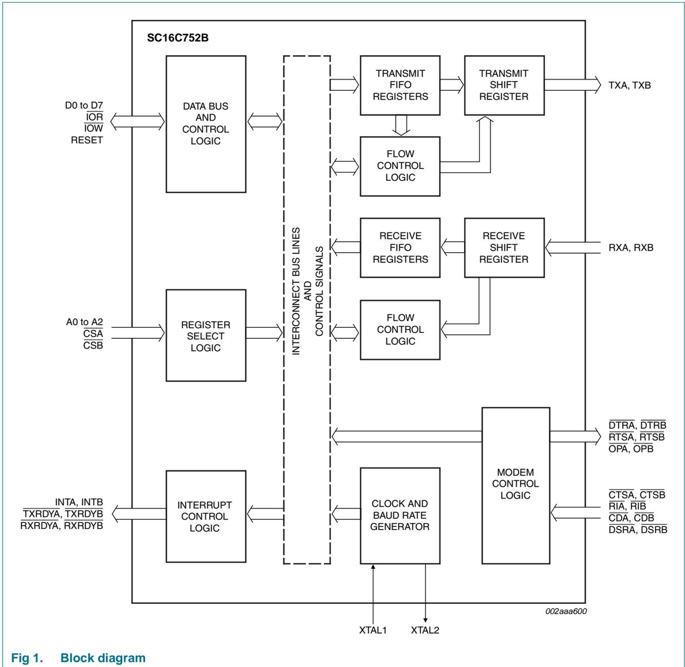
Fig 1. Block diagram
