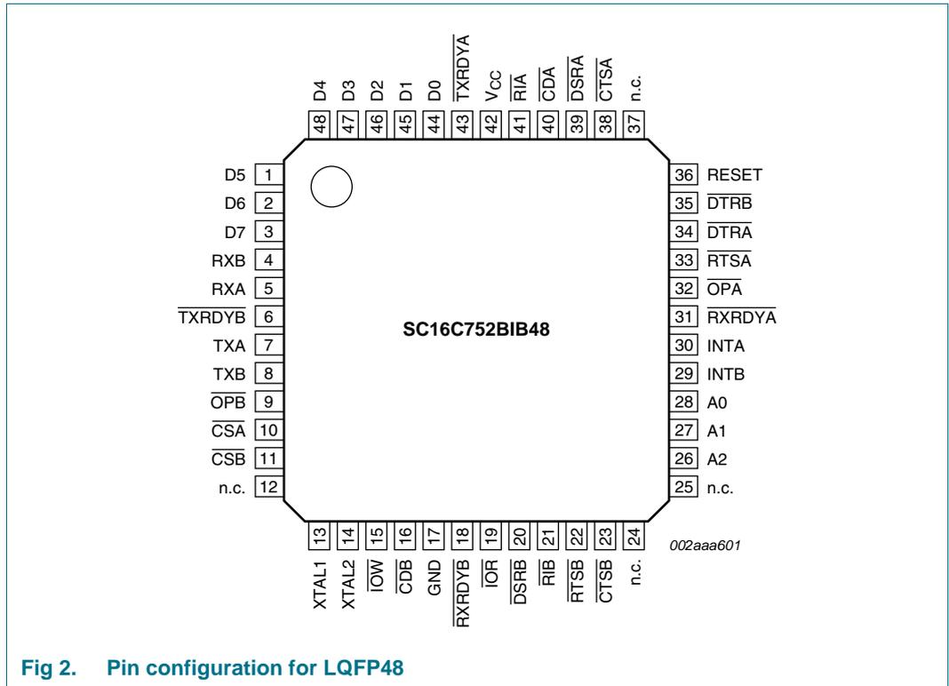
**Fig 2. Pin configuration for LQFP48**
