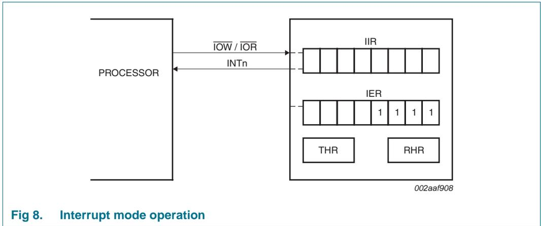
**Fig 8. Interrupt mode operation**
