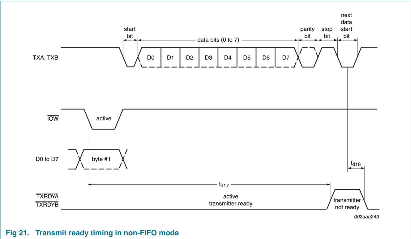
Fig 21. Transmit ready timing in non-FIFO mode
