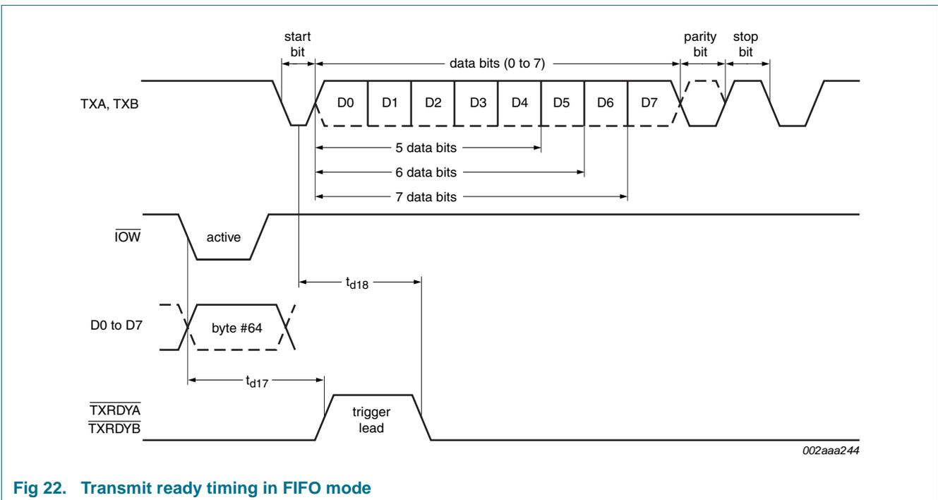
Fig 22. Transmit ready timing in FIFO mode
