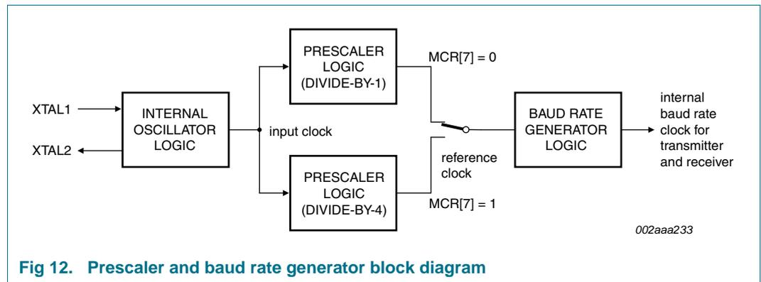
**Fig 12. Prescaler and baud rate generator block diagram**
