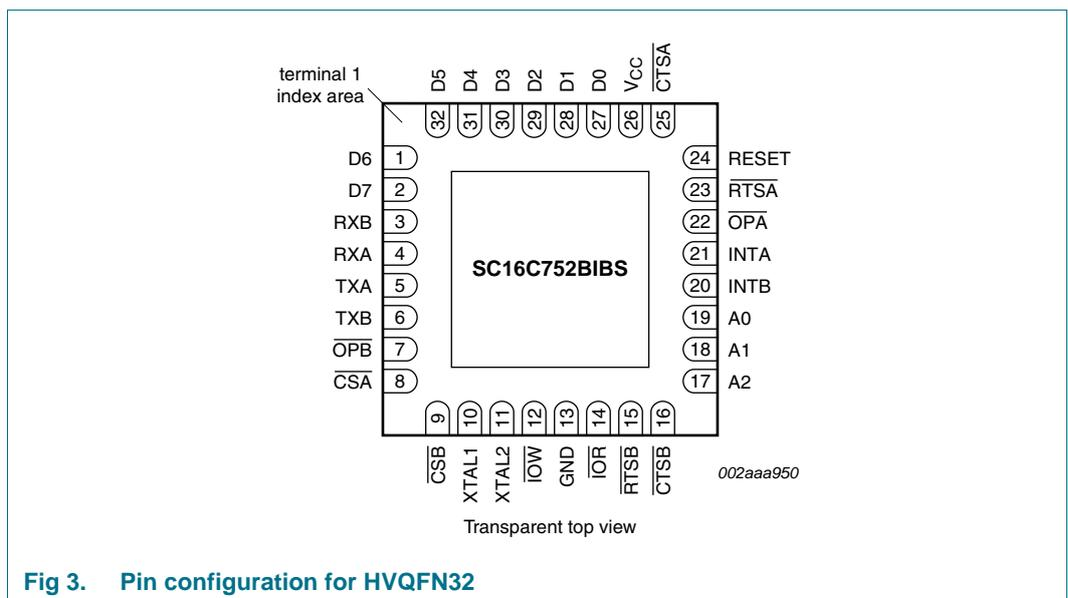
**Fig 3. Pin configuration for HVQFN32**
