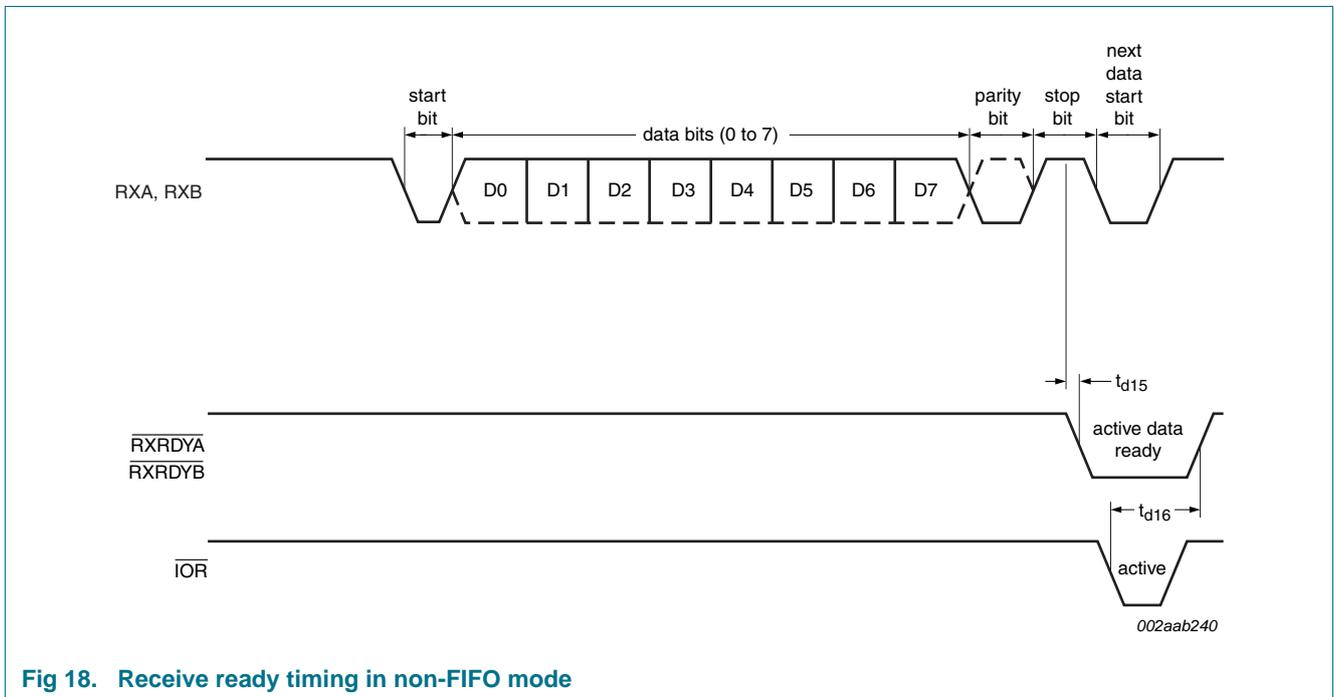
Fig 18. Receive ready timing in non-FIFO mode
