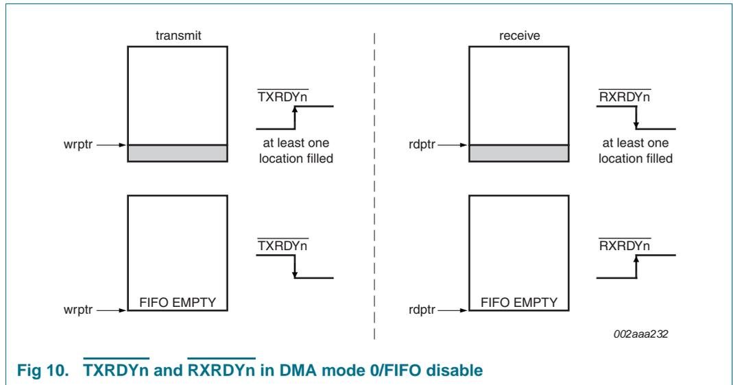
Fig 10.  $\overline{\text{TXRDYn}}$  and  $\overline{\text{RXRDYn}}$  in DMA mode 0/FIFO disable
