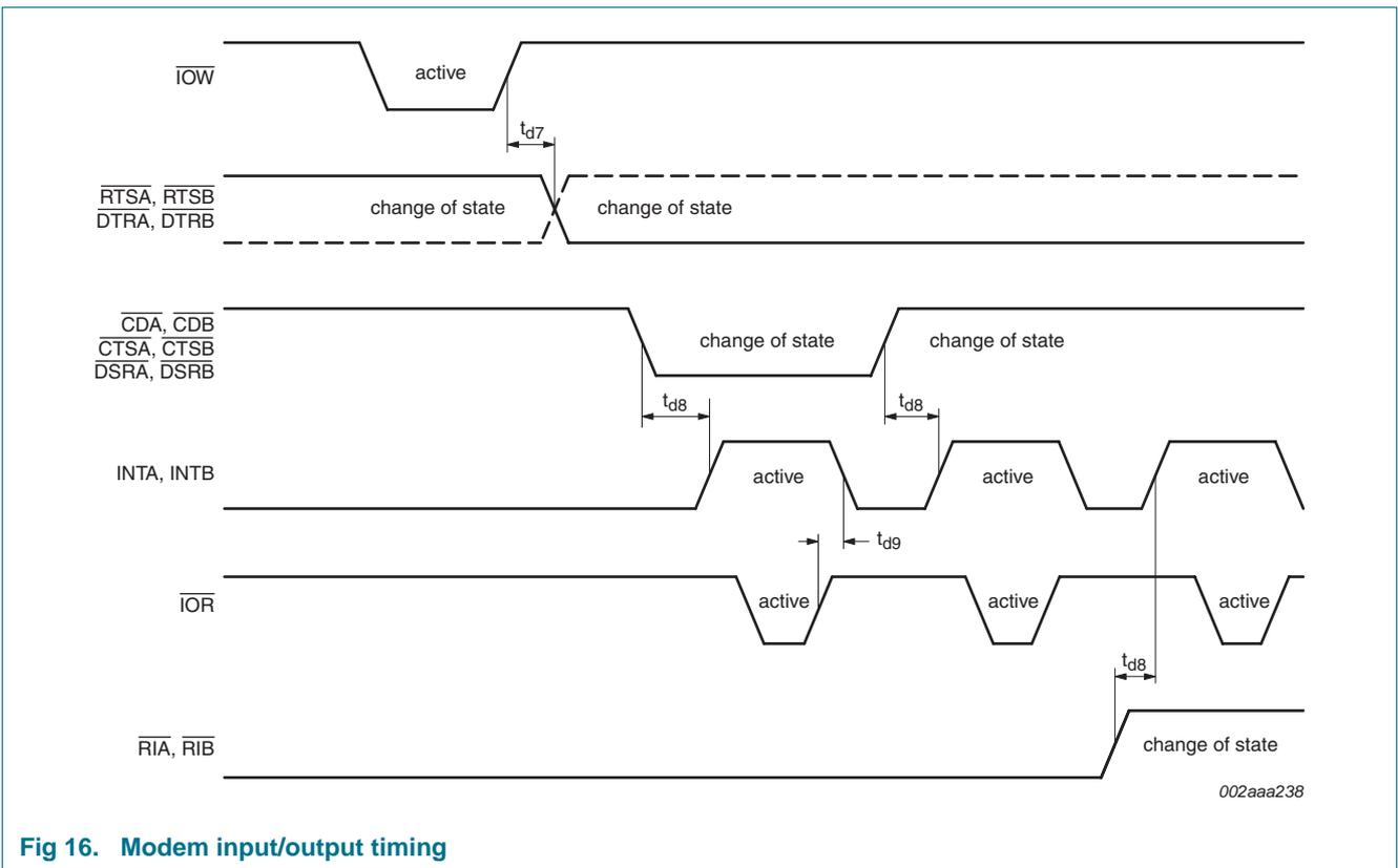
Fig 16. Modem input/output timing
