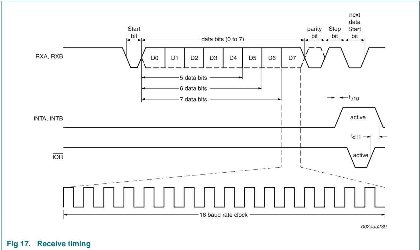
Fig 17. Receive timing
