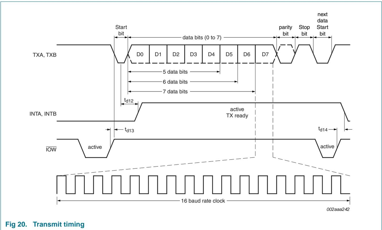
Fig 20. Transmit timing
