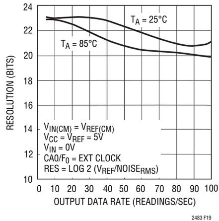
Figure 19. Resolution (Noise<sub>RMS</sub> ≤ 1 LSB) vs Output Data Rate and Temperature
