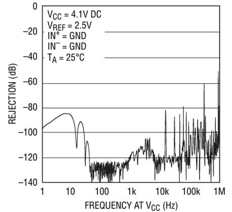
**PSRR vs Frequency at V<sub>CC</sub>**
