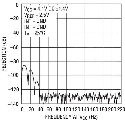
**PSRR vs Frequency at V<sub>CC</sub>**
