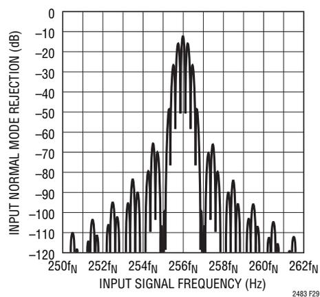
Figure 29. Input Normal Mode Rejection at  $f_s = 256f_N$
