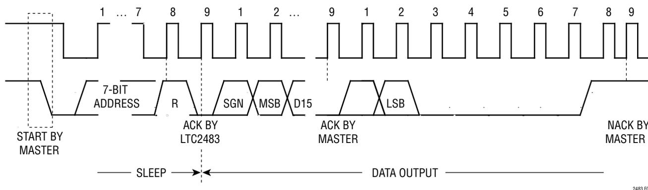
Figure 3. Timing Diagram for Reading from the LTC2483
