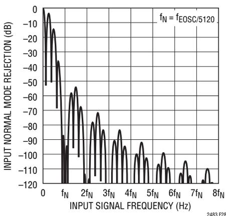
Figure 28. Input Normal Mode Rejection at DC
