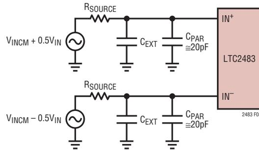
Figure 8. An RC Network at  $\text{IN}^+$  and  $\text{IN}^-$
