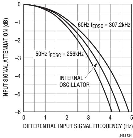
Figure 24. Input Signal Using the Internal Oscillator
