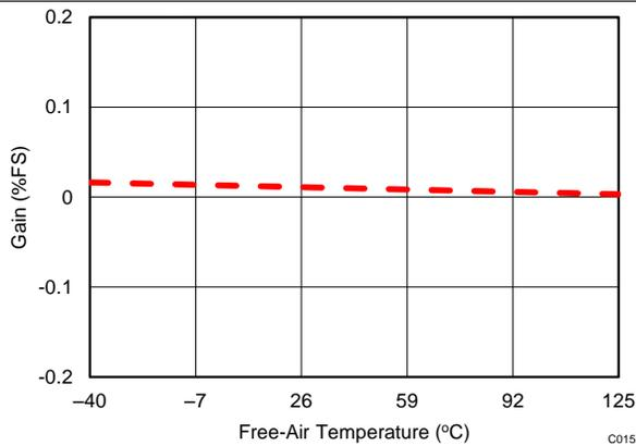
Figure 16. Gain Error vs Free-Air Temperature
