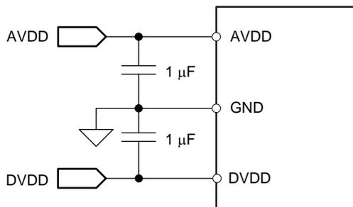
**Figure 46. Power-Supply Decoupling**
