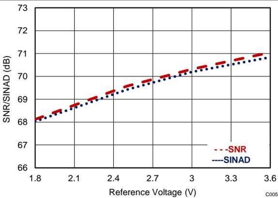
Figure 6. SNR and SINAD vs Reference Voltage (AVDD)
