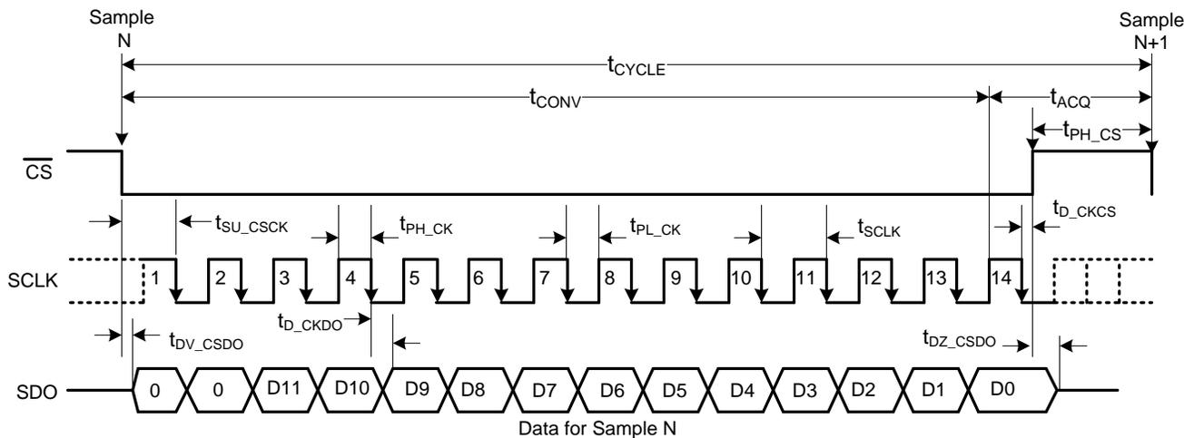
**Figure 1. Timing Diagram**
