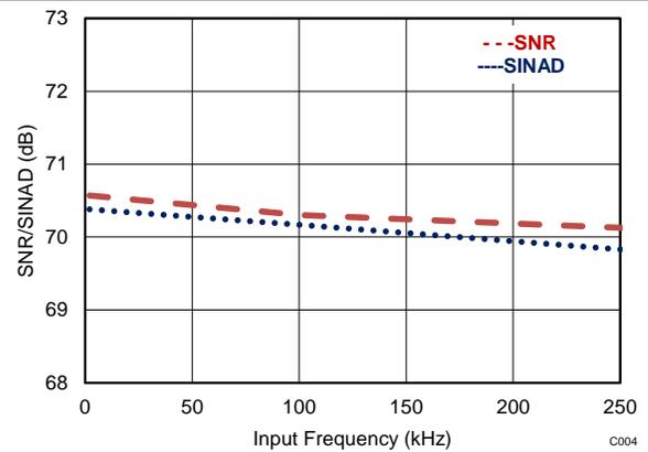
Figure 5. SNR and SINAD vs Input Frequency
