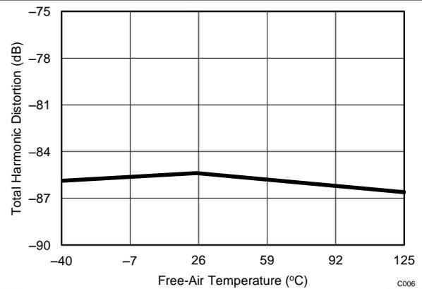
Figure 7. THD vs Free-Air Temperature
