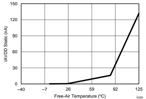
**Figure 29. AVDD Static Current vs Free-Air Temperature**
