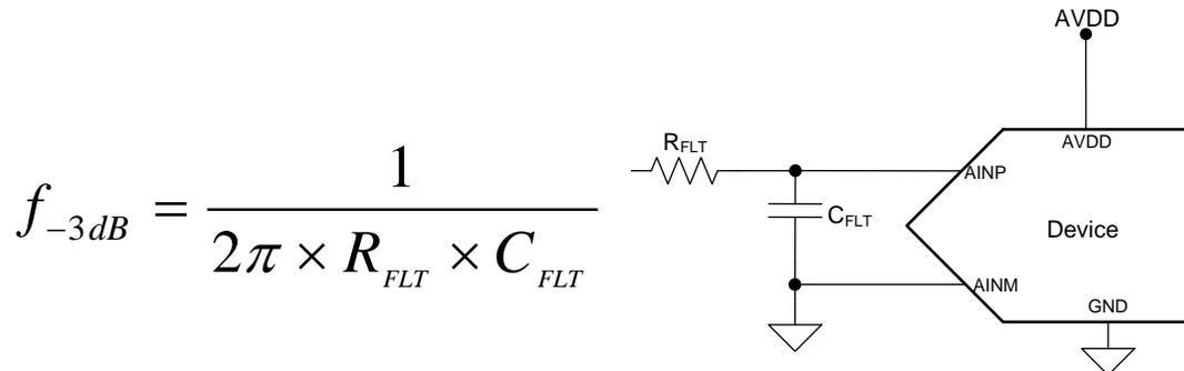
**Figure 39. Antialiasing Filter**
