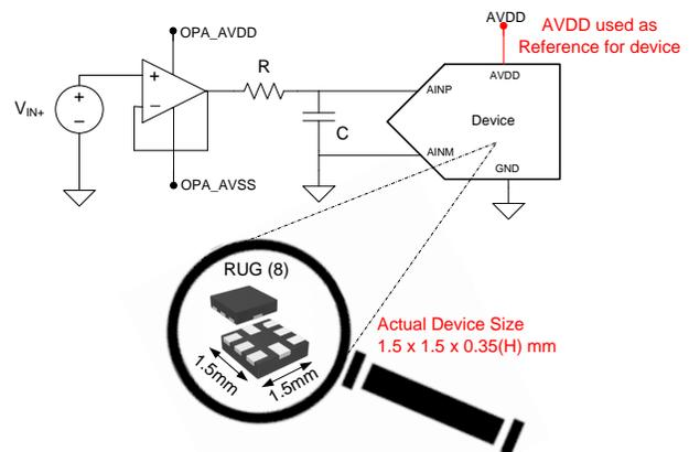
NOTE: The ADS7042 is smaller than a 0805 (2012 metric) SMD component.
