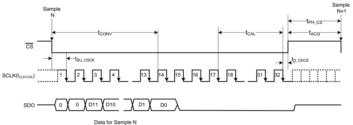
**Figure 37. Offset Calibration During Normal Operation Timing Diagram**
