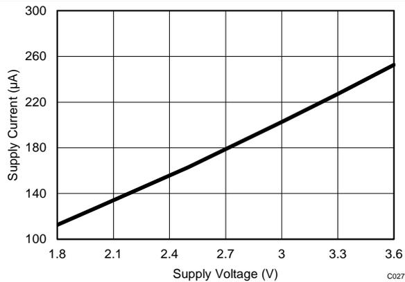
**Figure 28. AVDD Supply Current vs AVDD Voltage**
