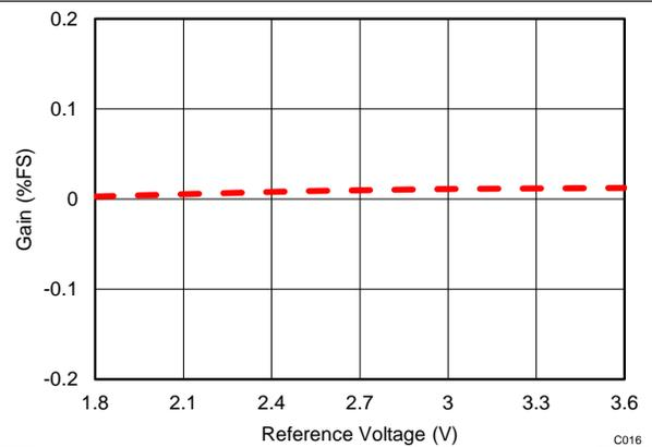
Figure 17. Gain Error vs Reference Voltage (AVDD)
