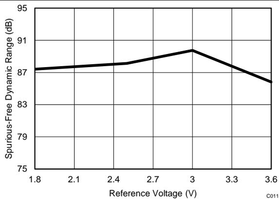
Figure 12. SFDR vs Reference Voltage (AVDD)
